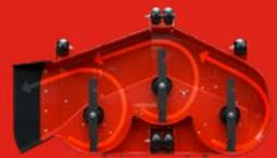
**TUNNEL CHAMBER** An advanced cutting chamber is formed by setting the blades back four inches from the front of the deck for less clumping and even grass dispersion.
