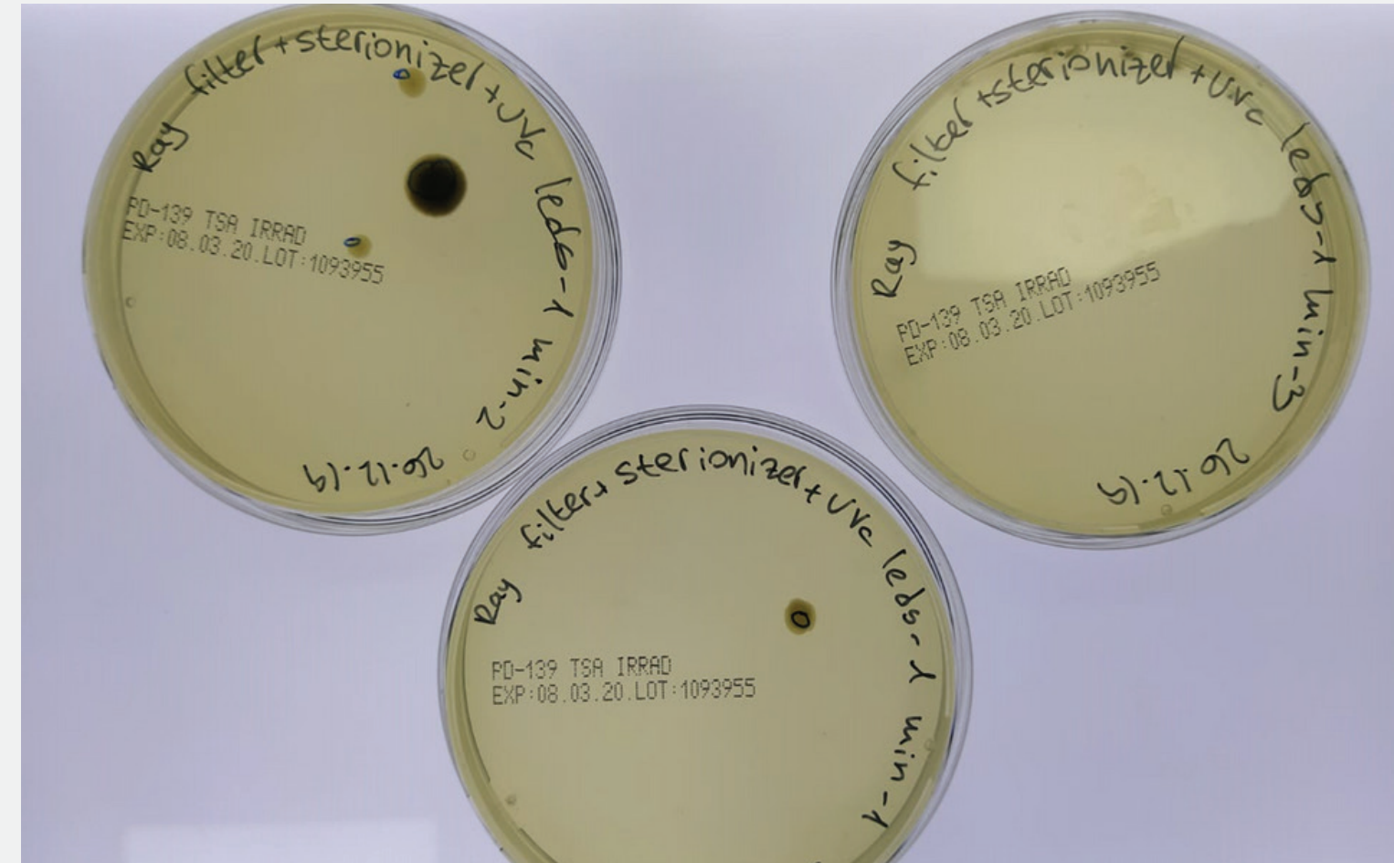
Incubation results of the Ray Filter™ + Sterionizer™ + UVC LEDs plates December 31st, 2019
