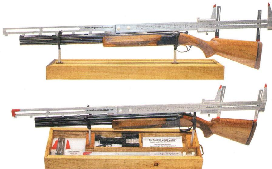
Made of lightweight aircraft aluminum, the Combo Gauge reads in both inches and metric and is compatible with a 23" extension that magnetically locks to the barrel—freeing both hands for precision work. With the optional second Drop Meter, users can measure multiple dimensions simultaneously, speeding up the process and enhancing accuracy.
