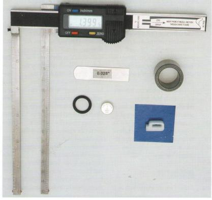
install a nylon fitting on the end of one probe and measure away. Nothing easier.
