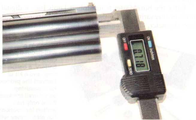
The digital readout on the BoreMaster gives you the actual diameter. You don't have to add or subtract the numbers from any nominal figure or calibration number; simply read the figure on the digital display.
