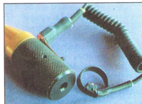
A battery-powered unit on the muzzle spud projects the laser beam. It's adjustable for windage and elevation.
