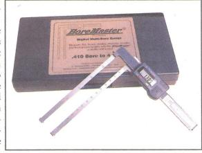
To check choke diameter, simply insert the probe fully and once the cylindrical bore reading is determined, the display is zeroed and the probe withdrawn to the choke and the amount of choke will be displayed on the readout.
