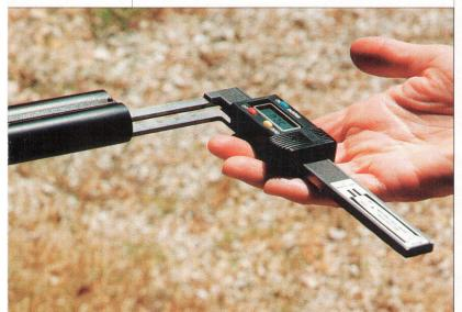
The Boremaster is a device that gives you digital readings of choke, chamber length, forcing cone and other measurements.
