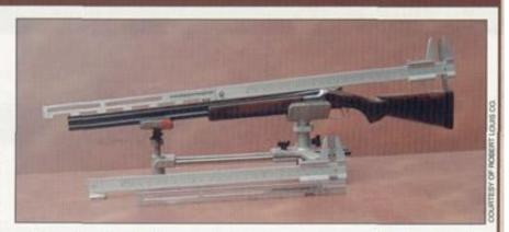
The Shotgun Combo Gauge can be used to measure everything from length of pull and drop to pitch.
