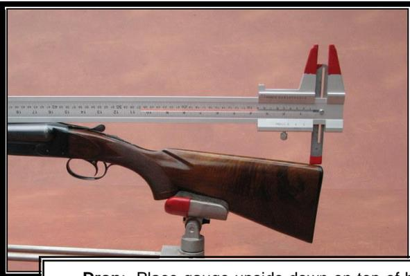
**Drop:** Place gauge upside down on top of barrel length and extend to point on stock at which you want to measure drop, usually at heel or at comb. Slide 6" drop meter down to top of stock.
