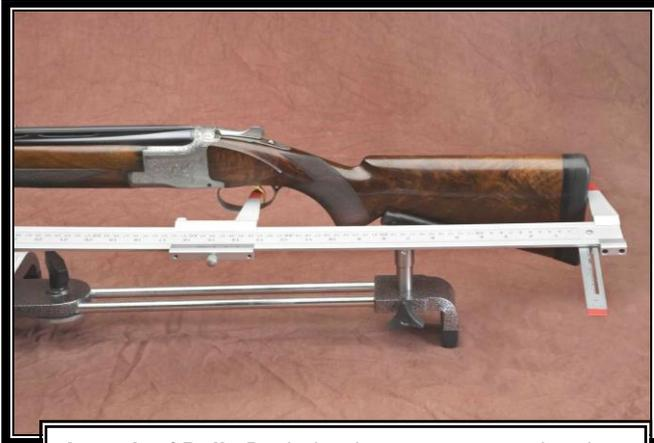
**Length of Pull:** Push the drop meter up so that the LOP is clear to be measured. Measure from inside trigger to end of stock. Read LOP at "0" mark.
