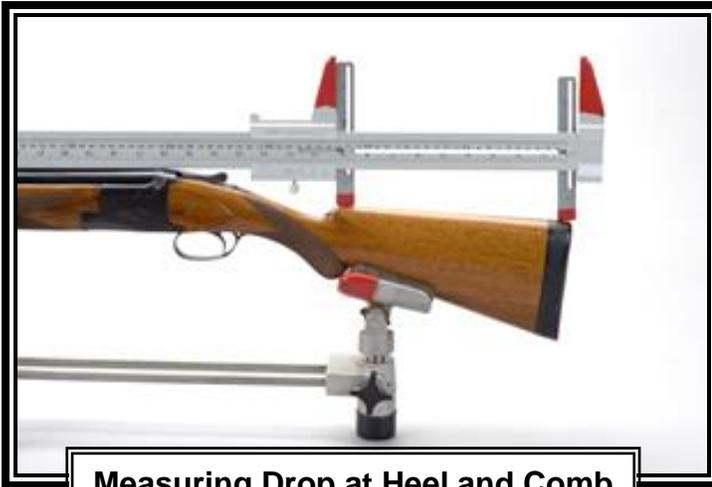
Measuring Drop at Heel and Comb Simultaneously
