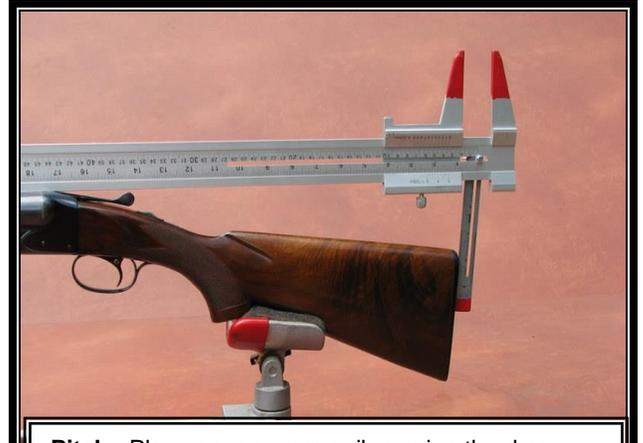
**Pitch:** Place gauge on gun rib moving the drop meter to the end of the butt plate. Extend drop meter to its total length and move parallel to the butt plate. Measure degrees of pitch with protractor.
