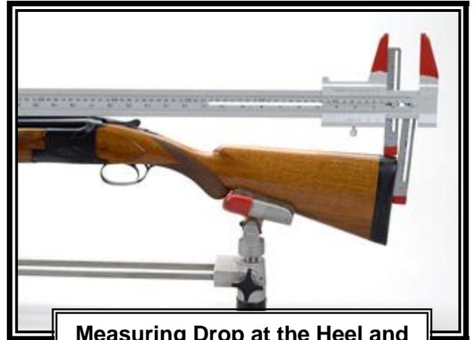
Measuring Drop at the Heel and Angle of Pitch Simultaneously
