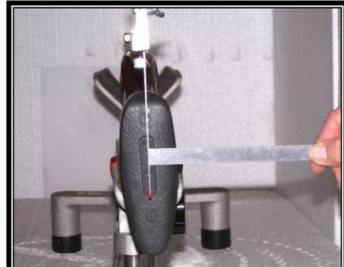
**Cast:** Mount Shotgun Combo Gauge with Extension on the center of gun rib. Set Drop Meter to low position parallel to the butt plate. Measure cast on or off with a ruler. Above gun shows "0" cast.
