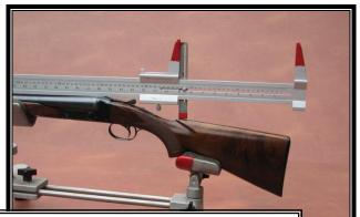
**Drop**: Place gauge upside down on top of barrel length and extend to point on stock at which you want to measure drop, usually at heel or at comb. Slide 6" drop meter down to top of stock.
