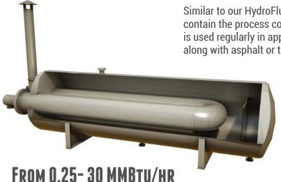
Similar to our HydroFlux IF, the DF (or Direct Fired) model does not contain the process coil, and is used to heat fluids directly. This model is used regularly in applications such as amine or glycol (TEG) reboilers, along with asphalt or tank heating.
