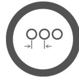
Tube spacing design is a critical component of heater design. THM uses the API guideline of '2D' spacing, which allows for the most even distribution of heat to the coils - ensuring you get the longest life possible out of your heat medium.
