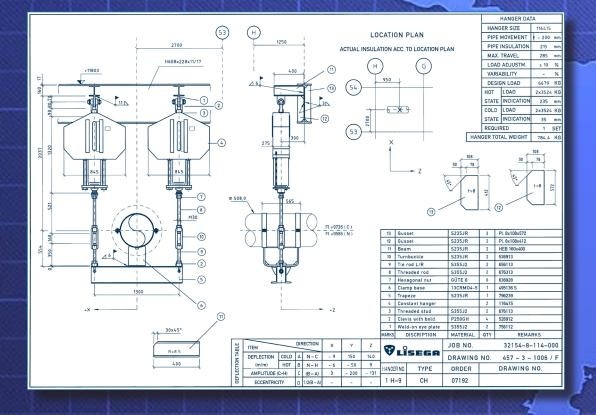
Individual support drawings detailed to your specifications can include loads, movements, bill of materials, installation dimensions, field weld sizes, offsets, location plan, and notes.
