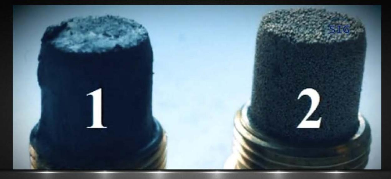
An example of coking of nozzles of burners operating on boiler – furnace fuel No.1 (Normal Fuel) and No.2 (Hydro fuel)
