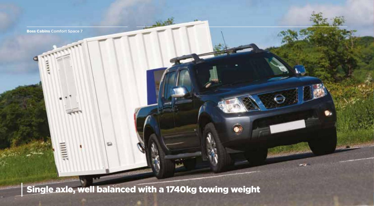
Single axle, well balanced with a 1740kg towing weight
