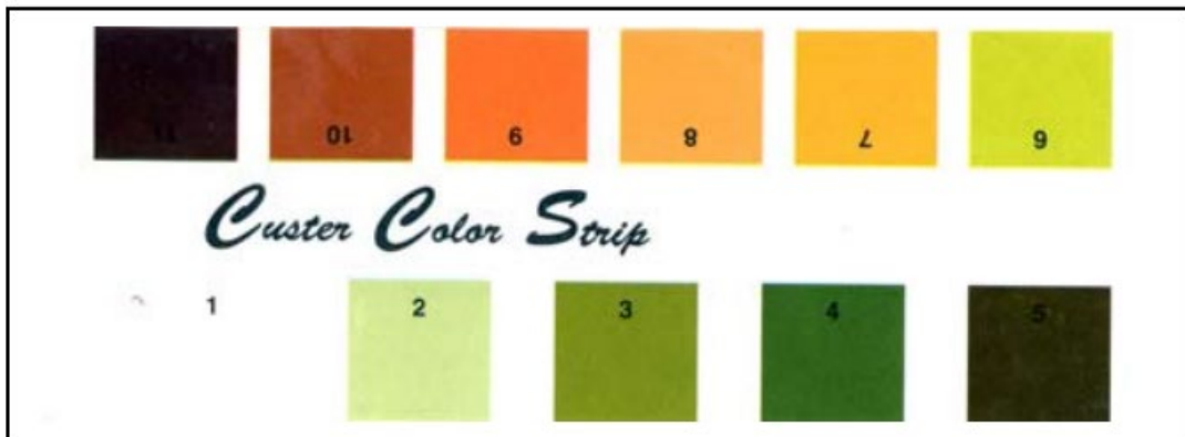
Figure 1. TCEH compared the color of the water on the Secchi disk (1 m) to the Custer Color Strip
