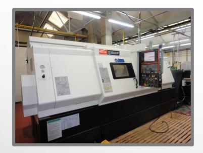
Large Capacity CNC Lathe capable of machining 700mm x 4000mm
