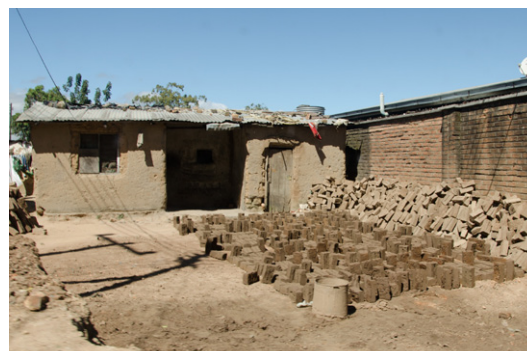
Production of adobe bricks in a peri-urban area near Blantyre. CC- Carmichael C.
