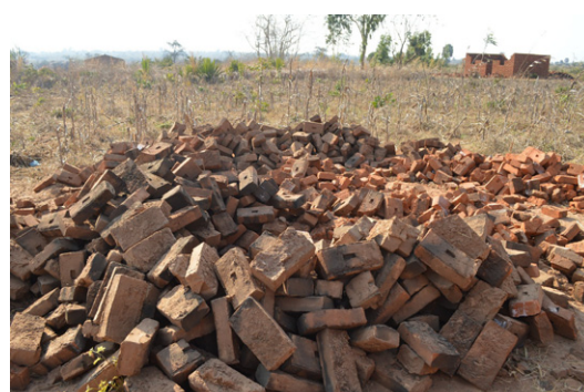
Burnt bricks have different qualities due to the varying intensity, time of firing and position in the clamps. Bricks in Muwanga, Chitipa. © Jon Twingi.
