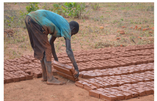
Bricks are hand moulded in wooden moulds. Brick production in Benga, Mchinji. © Jon Twingi.
