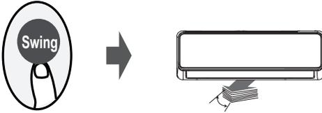
The horizontal louver will swing up and down automatically when pressing Swing button. Press again to make it stop.
