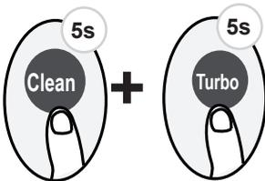
Press together **Clean** button and **Turbo** button at the same time more than 5 seconds to activate Lock function. All buttons will not response except pressing these two buttons for two seconds again to disable locking.
