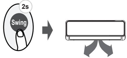
Keep pressing this button more than 2 seconds, the vertical louver swing function is activated. (Model dependent)
