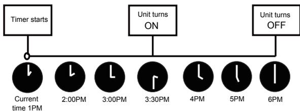
Example: If current timer is 1:00PM, to set the timer as above steps, the unit will turn on 2.5h later (3:30PM) and turn off at 6:00PM.
