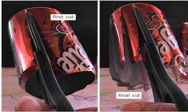
Fan each of the spokes outward and down. If you press your thumb against the bottom of each spoke before bending them with your other hand, it will help prevent the metal from crimping.
