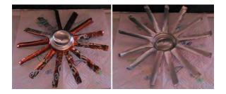
Cut away the excess metal at the end of each spoke where the can originally narrowed at the top.
