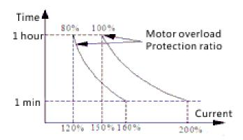
Figure FA-2 Motor overload protection coefficient setting
