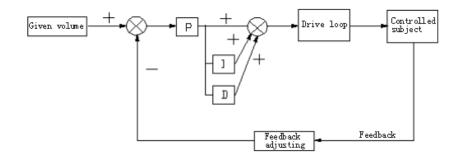
Figure F8-2 PID adjustment
