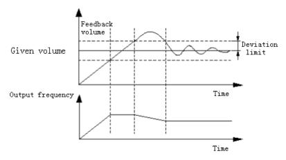
Figure F8-3 deviation limit diagram
