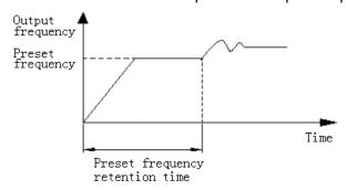
Figure F8-4 Closed-loop preset frequency operation diagram
