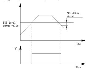
Figure F7-8 Frequency Level Detection
