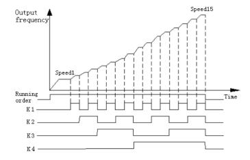
Figure F7-1 Multi-speed operation
