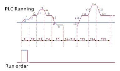
Figure F9-2 Maintaining the schematic after a single cycle of PLC
