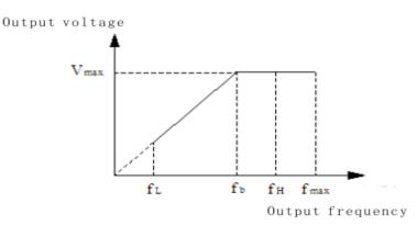
Figure F0-1 Voltage and Frequency Schematic
