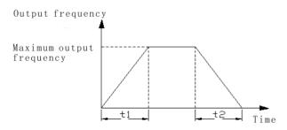
Figure F0-2 Acceleration time and deceleration time
