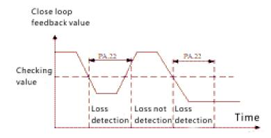
Figure FA-4 closed loop feedback loss detection timing diagram
