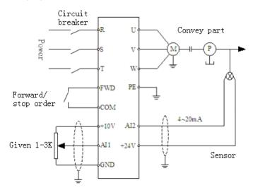
Figure F8-1 Analog Feedback Control System
