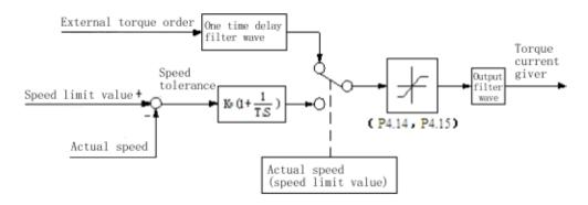
Fig. F4-2 Simplified block diagram of torque control
