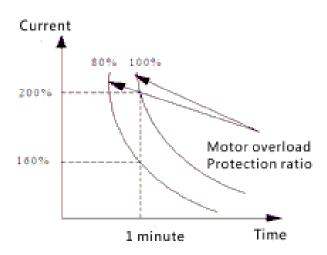
Figure FA-1 Motor overload protection curve
