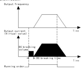
Figure F1-2 Starting DC braking
