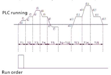
Figure F9-1 Stop after single-cycle PLC
