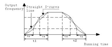
Figure F1-3 Acceleration and Deceleration of Straight Line and S Curve
