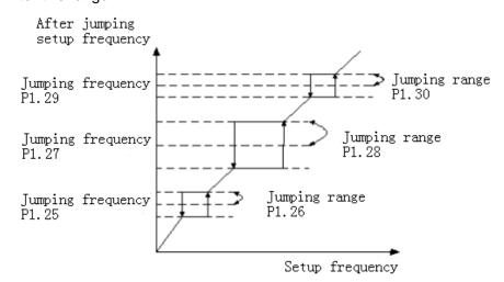
Figure F1-6 Jump frequency diagram
