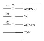
Figure F7-5 Three-wire control mode 2
