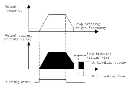
Figure F1-4 Shutdown DC Brake
