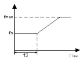
Figure F1-1 Startup frequency
