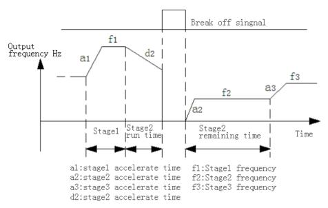
Figure F9-4 PLC starting method 1
