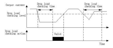
Figure FA-3 Load Drop Detection
