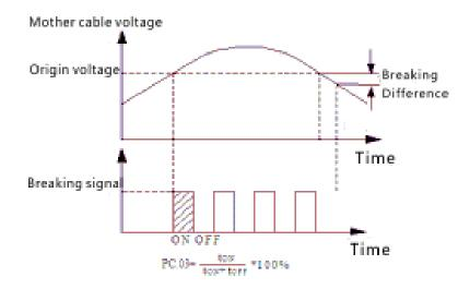
Figure FC-1 energy braking diagram
