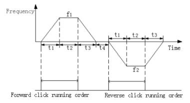
Figure P1-5 Jog operation diagram
