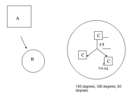
Figure 4. A) 50 ft square area to encompass a B) 24 ft in radius circular plot and layout of C) three  $1m^2$  parcels
