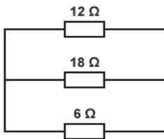
(ii) Redraw the above circuit in such a way that the resultant resistance is 22 ohms. Show the calculation.
