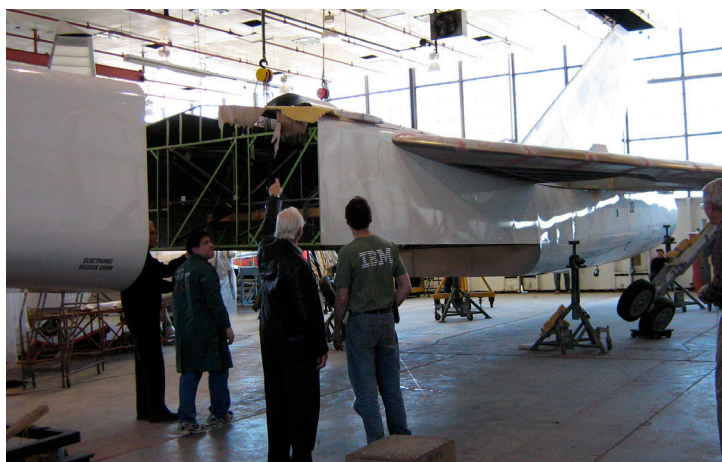
Claude Sherwood oversees the joining of the Arrow cockpit and fuselage, April 8, 2006.
