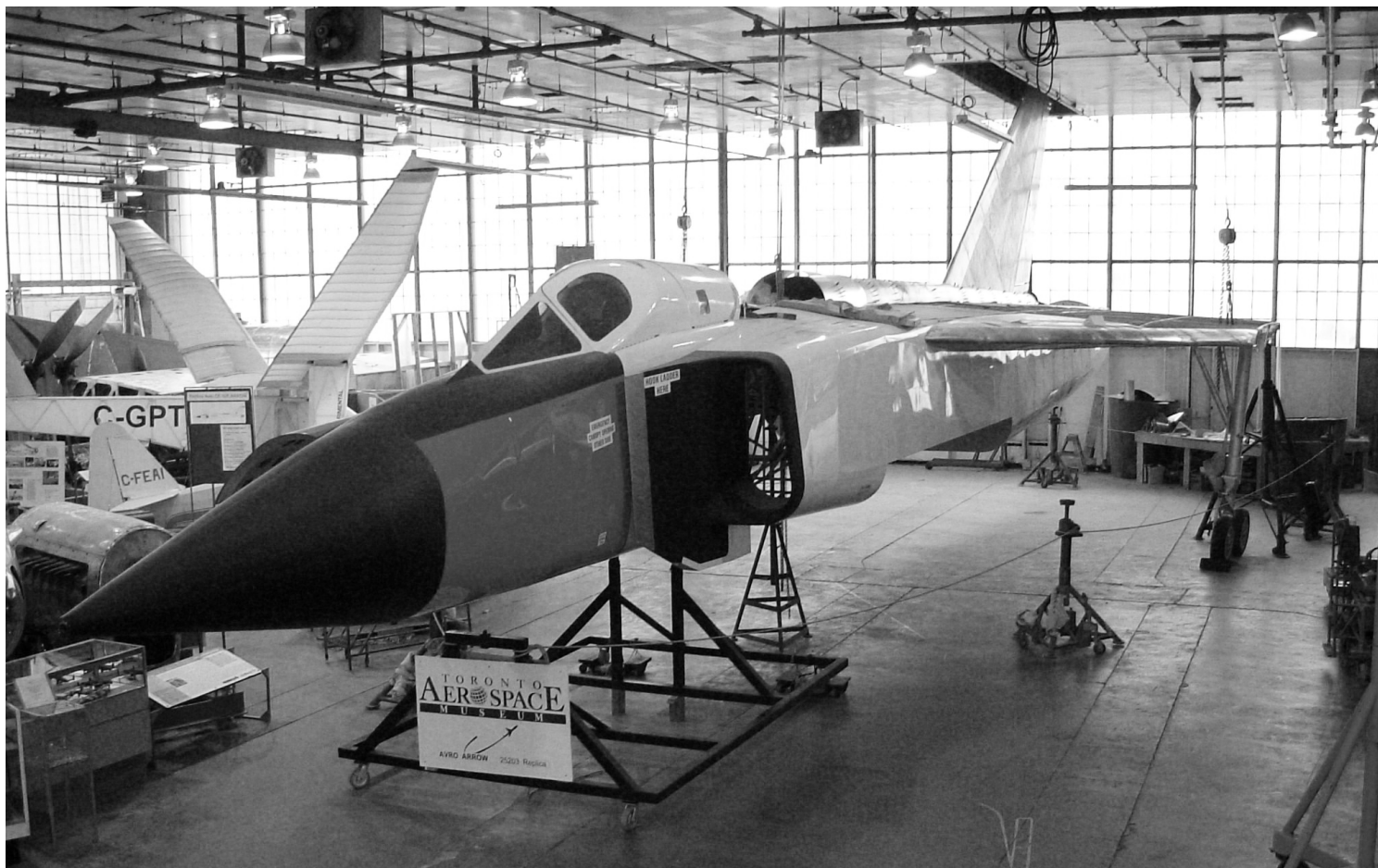
Arrow replica on April 10, 2006 after the fuselage was mated together and the main landing gear installed. The museum hangar was built by DHC in 1941-1942 as the paint shop for Avro Anson II trainers and DH 98 Mosquito fighter-bombers. Photo Ken Swartz.
