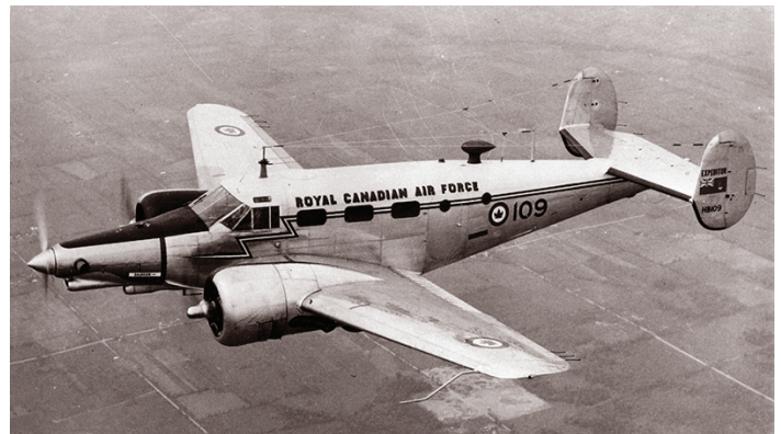
The RCAF C45 Expeditor - Modified Test Vehicle for the PT6 Engine Photo Courtesy - P&WC.
