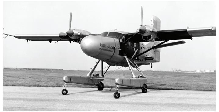
DHC Otter modified for STOL Research. Photo - DHC.
