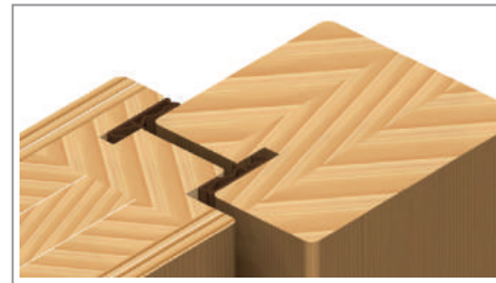
Detail – double sealing
