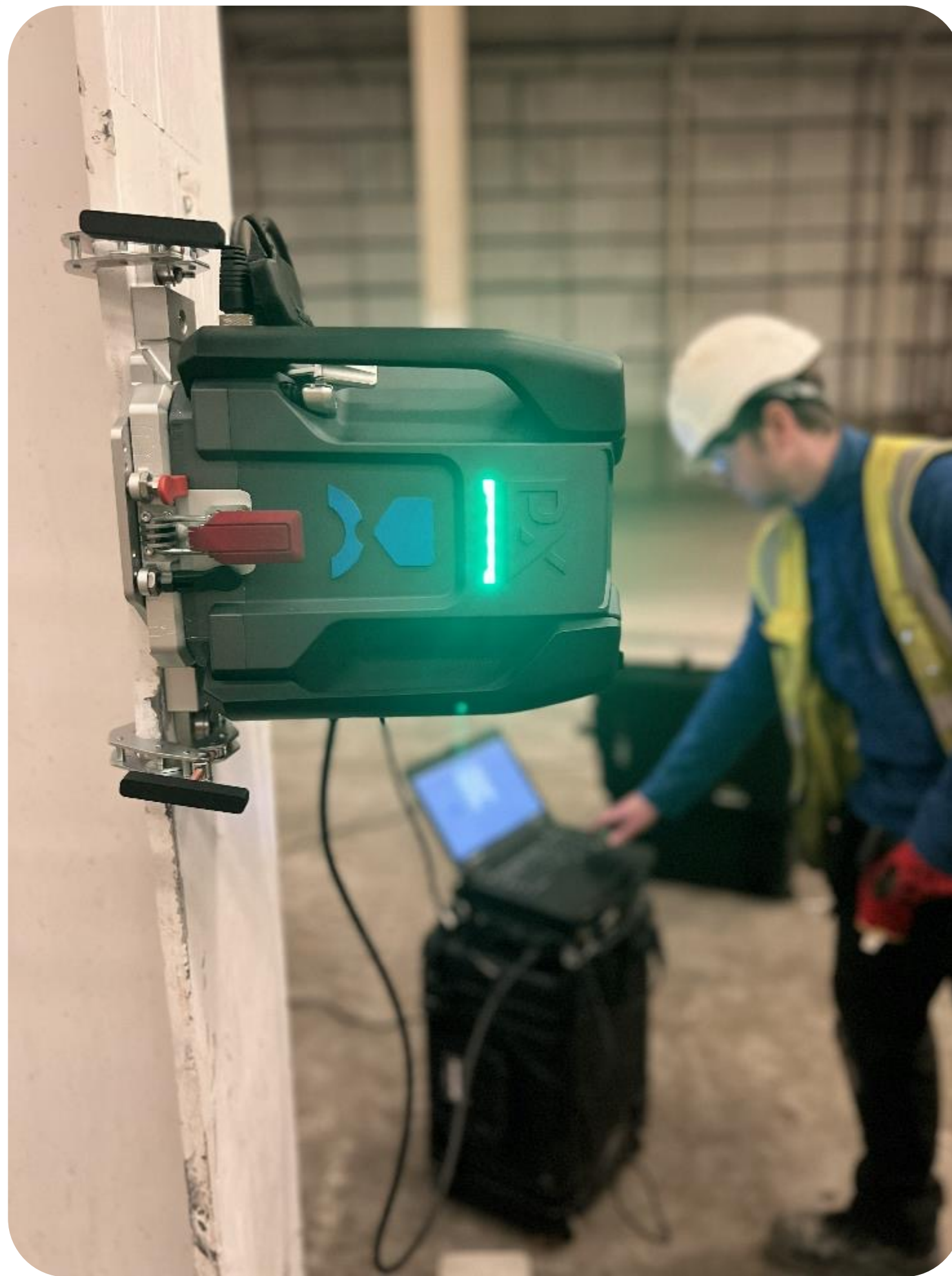
Sandberg Technician operating the PLX Indenter on site.
