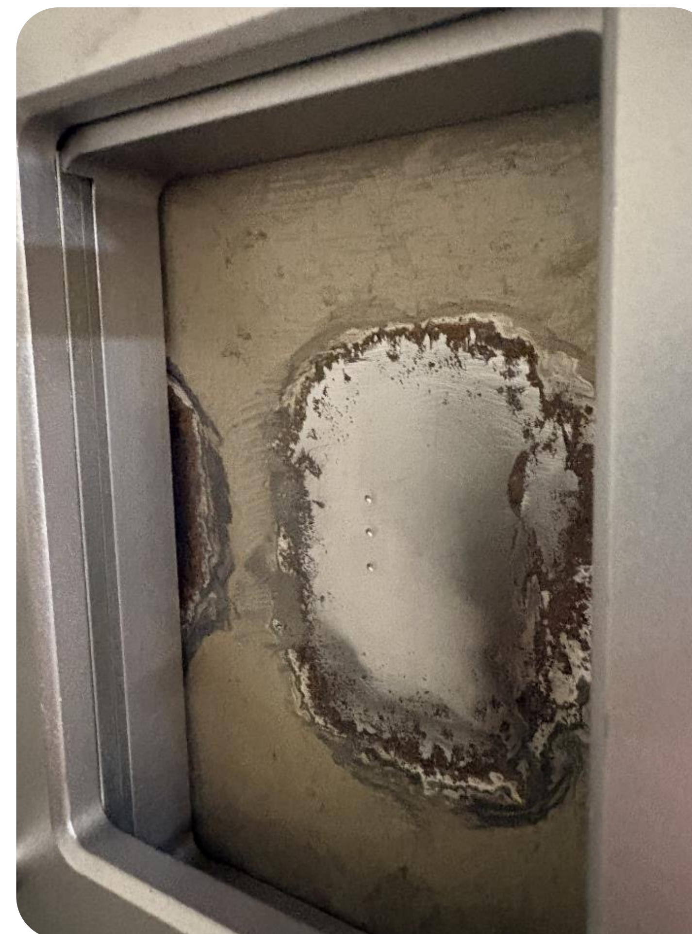
Indents made by PLX Portable on site.
