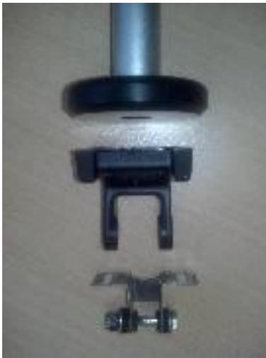
For “conventional” transducers from Humminbird or Lowrance, the Mounting disk shown is supplied.
