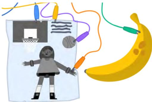
Connect different pieces of your drawing to alligator clips. Make sure the conductive pieces don't overlap, so only one key is registered as pressed at a time.
