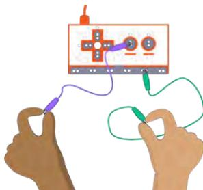
One person holds the alligator clip connected to the keyboard key. The other holds the clip connected to EARTH.
