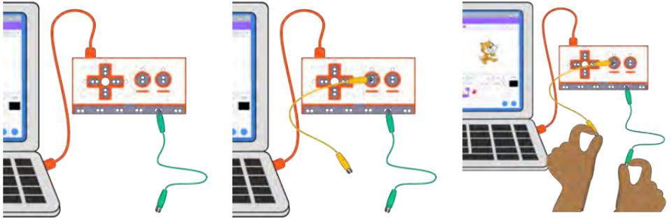
3. Connect an alligator clip to any set of holes along the “EARTH” strip on the bottom of the board.
