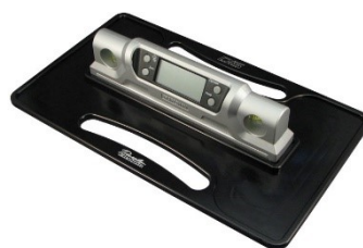
Figure 7: Official measuring device to check saddle inclination
