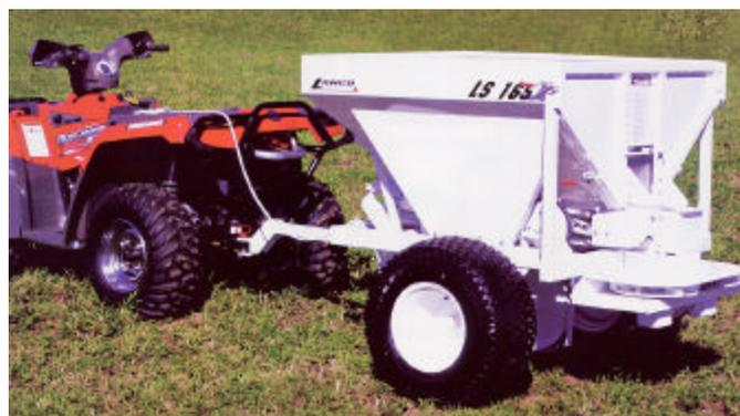
Fertilizer Spreader: For ATV and small utility vehicles. Can spread fertilizer, lime, sand & salt. Stainless steel conveyor.
