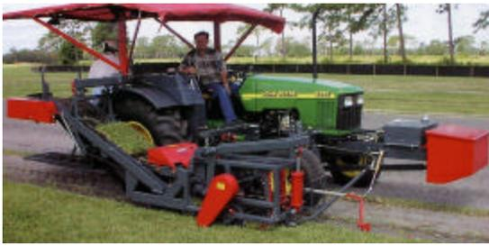
Sod Harvester - Slabs
