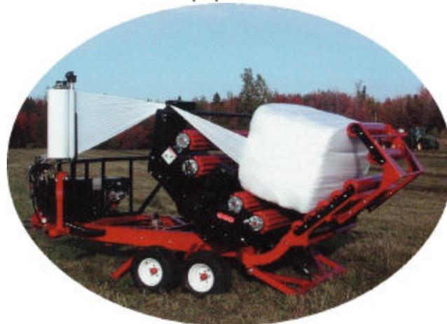
Square Bale Wrapper: Wraps big square bales up to 72" long. Includes hydraulic bale dumper, automatic cut & hold.
