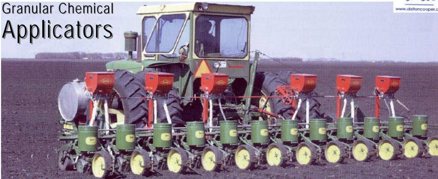
Row Crop Applicators: Applies granular herbicide, insecticides while planting, cultivating. Precision cam gauge metering. Stainless steel bottom slides control openings. Tool bar mounting. Ground drive or 12-volt motor. Hopper capacity: 100, 45, 30, 20 pounds.
