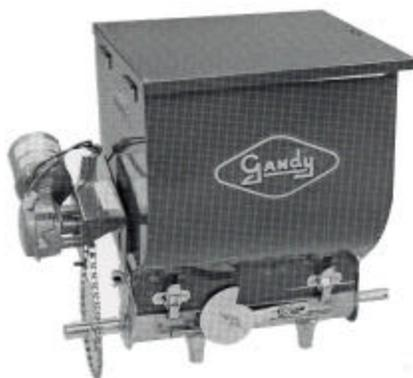
Forage Preservative Applicators: Applies granular preservatives during baling or harvesting. 12-volt motor drive. Poly PDA units have convenient In-Cab rate control.
