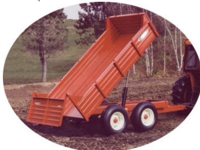
Dump Trailers: 1.5 to 12 ton models. Rear dumping. Highway or off-road models. Tandem wheels. Double action cylinders.
