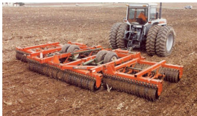
**Pulvi-Mulchers (Roller Harrows):** Creates clod-free seedbed in one pass. Front rollers & spring teeth crush clods & rear rollers create firm seedbed. Ductile iron wheel is 2.5 times stronger.
