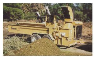
Mini Grinder: Grinds variety of wood wastes (tree branches, palm fronds, pallets...) to small particles. Hammermill action.
