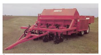
Front view: showing special coulters to cut thru residues.
