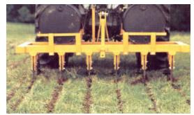
Pasture Renovators: Revitalizes pasture by allowing water & fertilizer to root zone. 17" coulter blades + 17" slicer shanks.
