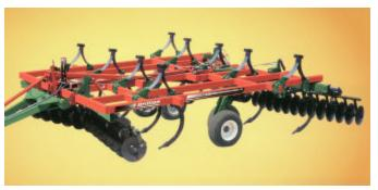
Land Commanders: Cuts thru heavy residues & works on soil down to 18" deep. Breaks up hard pan & promotes root growth. 11 to 20-ft width. 39" under frame clearance for easy trash flow.
