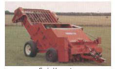
Sod Harvester - Slabs
