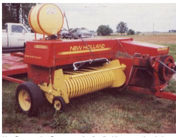
Hay Preservative Sprayers: Applies liquid preservative during baling or harvesting. 3 nozzle boom covers pick up width on baler. Optional In-Cab control for adjusting pressure from cab.
