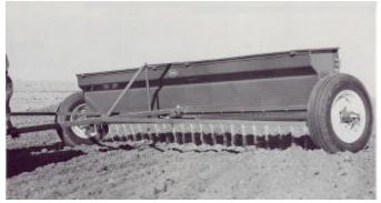
10T Fertilizer Spreaders: Precision drop spreaders. Cam gauge metering & Stainless steel bottom. 6 to 12-ft. width.
