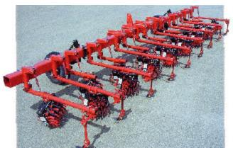
Rolling Cultivators: Versatile tillage tool. Builds and mulches bed. Can handle residues. Most accurate row crop cultivator in any soil.
