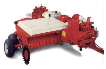
Pull Type Baler: Widest pick-up width (76"). Produces high-density bales which can be stack handled & re-handled.
