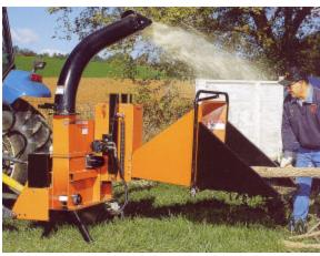
Brush Chippers: Chips wood branches up to 8" in diameter. Reduces solid waste and produces wood chips and mulch.
