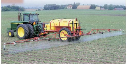
Large Row Crop Trailer Sprayers: 300 to 1000 gallon capacity elliptical tank. 45 to 60-ft truss boom. 18 or 20" spacing nozzles. Hydraulic lift & fold wings. Raven control. Roller pump or centrifugal pump. Optional foam marker, hand gun, Raven GPS light bar.
