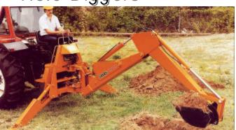
Backhoe attachments: Mount on tractor 3-pt hitch. Dig 6, 7, 9 or 10-ft deep. Hydraulic drive. Joystick control.
