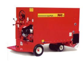
Motorized Feed Carts: Accurately feeds cattle, hogs in dairy barns. Reliable Honda engine & hydrostatic drive, easy controls, 6-ply tires. front, side or high discharge.
