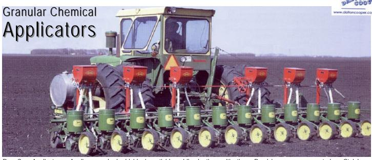
Row Crop Applicators: Applies granular herbicide, insecticides while planting, cultivating. Precision cam gauge metering. Stainless steel bottom slides control openings. Tool bar mounting. Ground drive or 12-volt motor. Hopper capacity: 100, 45, 30, 20 pounds.
