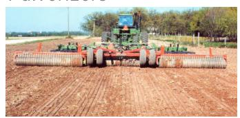
Pulverizers: Pulled behind disc or field cultivator. Creates ideal seedbed by firming up the seedbed (for uniform planting depth). Eliminates air pockets for good soil to seed contact.
