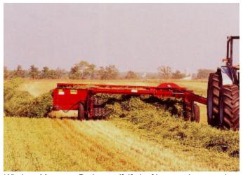
Windrow Mergers: Reduces alfalfa leaf losses when merging few windrows into one for high volume harvesting / baling.
