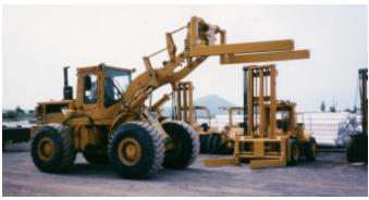
Hay Squeeze Attachment: Attaches to a Loader or a large
