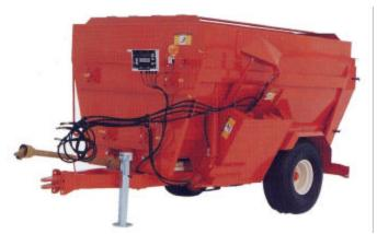
TMR Mixers: 4 auger mixing system. Mobile or stationary models. Heavy planetary gear box. 4 weight bar electronic scale.
