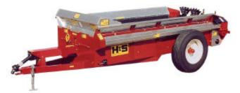
Heavy Duty Manure Spreaders: 235 or 310 bushel models. Patented 2 speed enclosed gear box, 16,000-lb tensile strength T-rod apron chain. Optional hydraulic endgate. Shear bolt.
