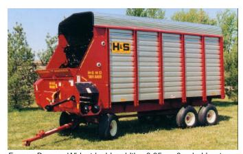
Forage Boxes: Widest inside width - 2.25m. 3 spiral beaters. Progressively faster top to bottom beaters deliver smooth even flow to cross conveyor. Twin auger conveyor or chain & slats.
