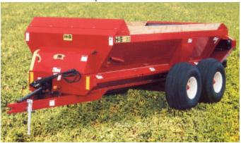
All Purpose Spreaders: Spreads hard, liquid or semi-liquid manures. Features V-tank, hydraulic variable speed twin augers, PTO driven inside shredder beater & rear expeller auger, hydraulic rear endgate. Very versatile manure spreader!
