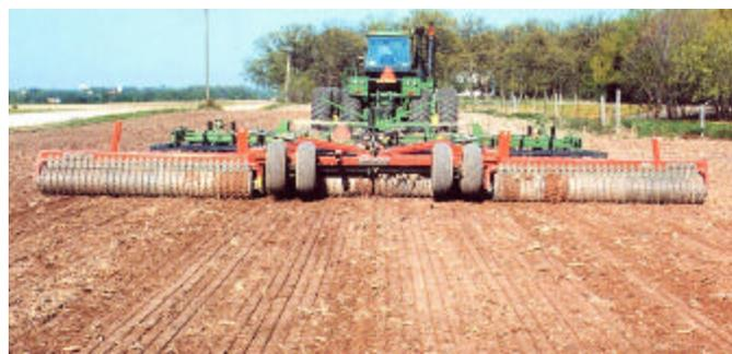
**Pulverizers:** Pulled behind disc or field cultivator. Creates ideal seedbed by firming up the seedbed (for uniform planting depth). Eliminates air pockets for good soil to seed contact.
