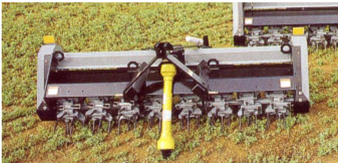
Front view of AGRI-vator showing the vibrating tines (rotors).
