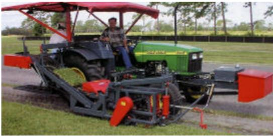
Sod Harvester - Slabs
