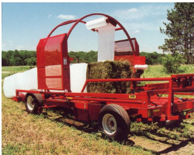
In-Line Bale Wrapper: Efficiently wraps round bales or big square bales one after another. Automatic & self-propelled.
