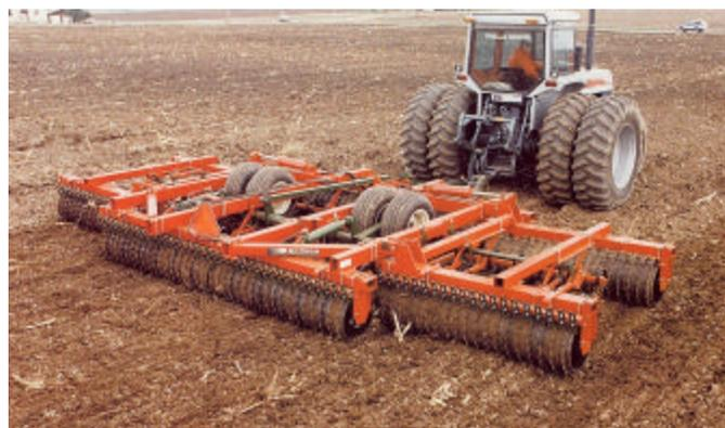
**Pulvi-Mulchers (Roller Harrows):** Creates clod-free seedbed in one pass. Front rollers & spring teeth crush clods & rear rollers create firm seedbed. Ductile iron wheel is 2.5 times stronger.
