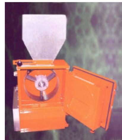
Hammermills: Shreds Grains for feeding. Can be mounted directly over mixer or on discharge auger.
