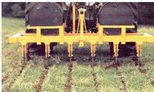
Pasture Renovators: Revitalizes pasture by allowing water & fertilizer to root zone. 17" coulters blades + 17" slicer shanks.
