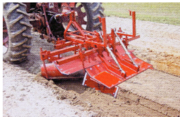
Bed Shaper: Gathers soil & roll it together. Large curved wings w/cutting blades. Options: fertilizer attachment, mulch layer.
