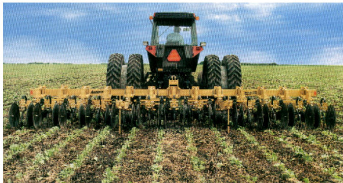
Row Crop Cultivators: Single shank row crop cultivators, Adjustable row crop cultivators, vegetable row crop cultivators, Delta row crop cultivators, high residue row crop cultivators.
