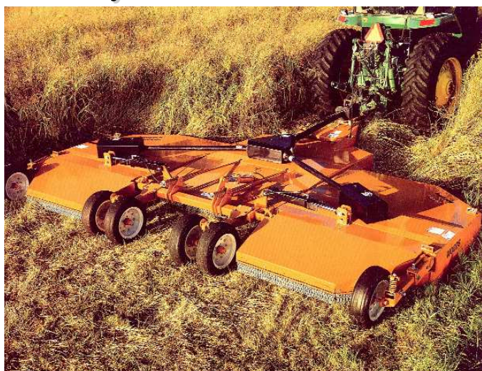
Folding Wing Rotary Cutters: Heavy duty gearbox, heavy duty slip clutches, dual spring loaded wheels, hydraulic folding wings.
