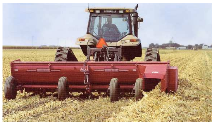
Flail Windrowers: Shreds & windrows in one pass. Cross auger forms uniform windrows for baling or stacking. 15-ft width.
