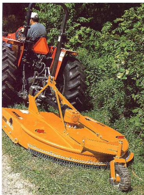
Heavy Duty Rotary Cutters: High speed single spindle cutter. Heavy duty 150-hp gearbox. Category 5 drive line. High capacity slip clutches. 60", 72" or 84" cutting width.
