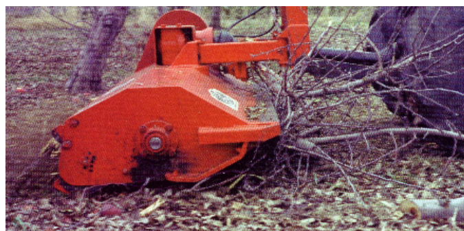
Orchard Shredder: Extra heavy duty flail shredder. Tractor 3-pt hitch or pull type. Offset models available. 4 to 9 ft width.
