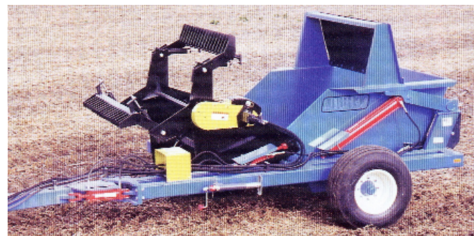
Rock Pickers: Hydraulic powered continuous rocking picking machine. Hydraulic dump. 48" or 60" pick up width.
