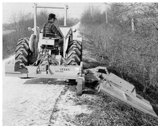
Ditch Bank Mower: Cuts grass and brushes on hard to reach road shoulders & ditchbanks. 5 or 6-ft cutting width.
