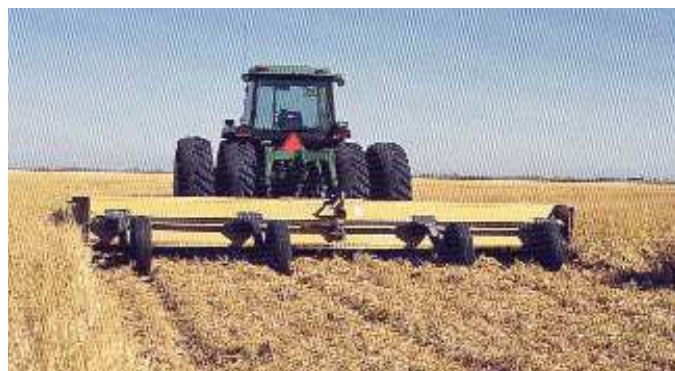
Flail Shredders: Shreds any crops on field. For non-row crop applications. Leaves virtually no strips. 12 to 24-ft width.
