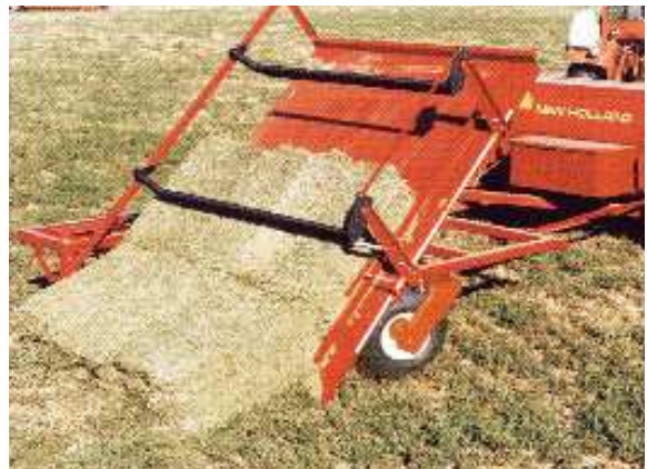
Bale Accumulator: Accumulates 10 bales. Automatic dumping. Attaches directly behind a baler.
