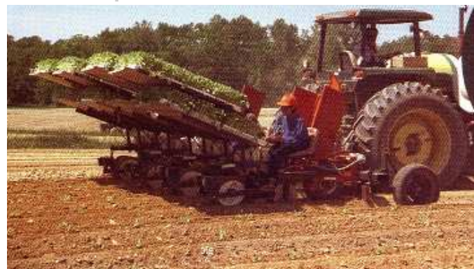
Rotary One Transplanters: For planting greenhouse tray plug plants. 6 rotating plant cups. Plants 70 plants per minute.
