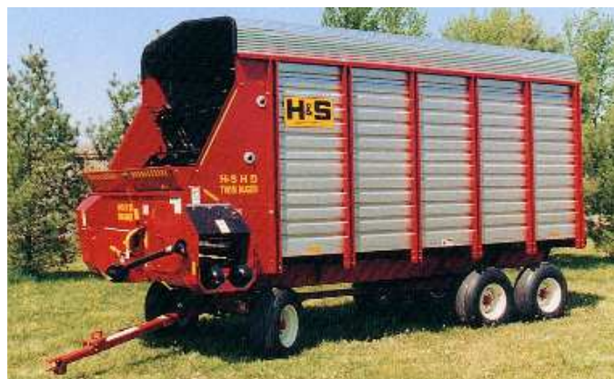
Forage Boxes: Widest inside width - 2.25m. 3 spiral beaters. Progressively faster top to bottom beaters deliver smooth even flow to cross conveyor. Twin auger conveyor or chain & slats.
