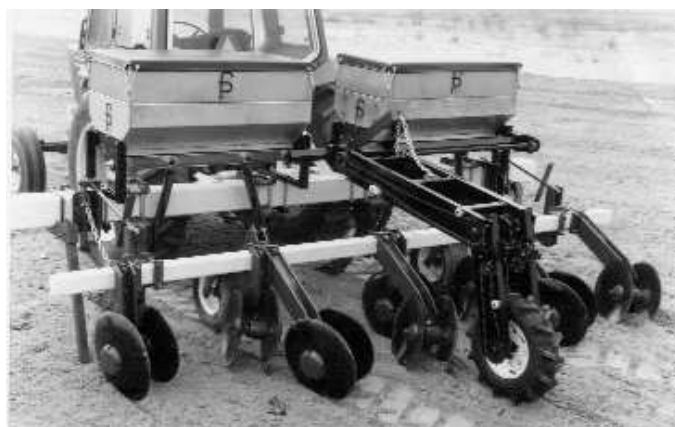
Fertilizer Applicators: Precisely places fertilizer during planting or cultivating. 500 or 1000-lb. hopper. Ground or hydraulic drive.
