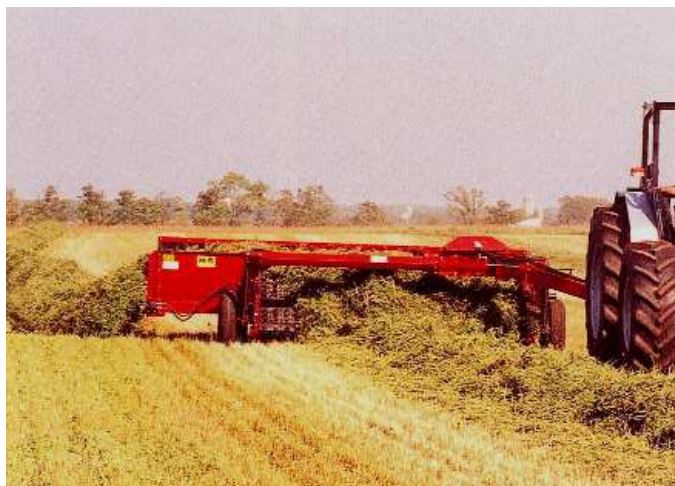
Windrow Mergers: Reduces alfalfa leaf losses when merging few windrows into one for high volume harvesting / baling.
