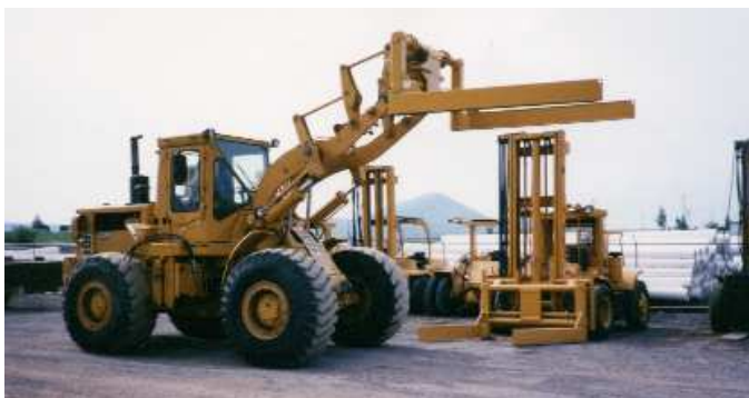
Hay Squeeze Attachment: Attaches to a Loader or a large Forklift. Lifts 8x8 bale stacks. Loads trucks in minutes. Lifts up to 14 to 20 feet. Fork length 96", squeeze opens to 102", closed 65". Weight 3300 lbs.
