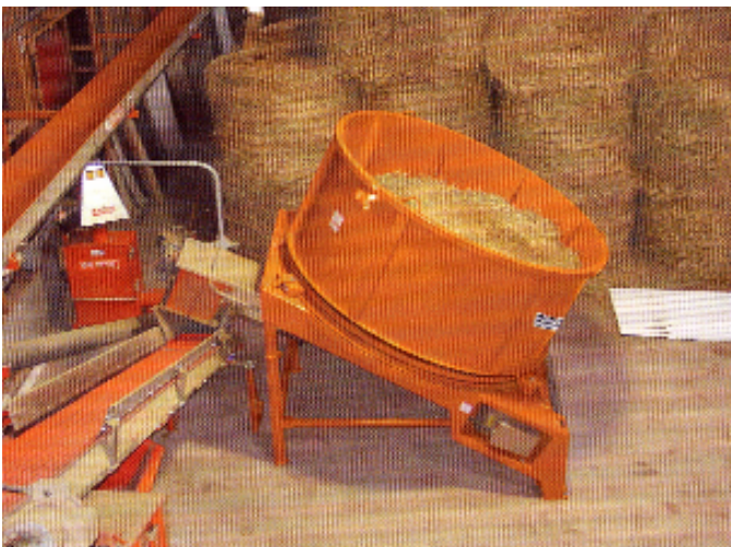
Stationary Bale Chopper: Shreds round or big square bales in door for feeding. Sharp knives require little electrical power.
