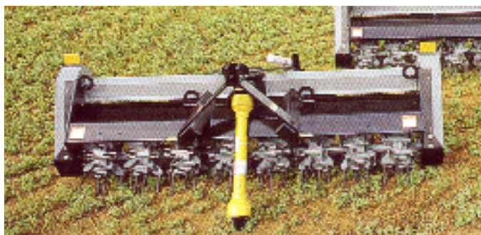
Front view of AGRI-vator showing the vibrating tines (rotors).
