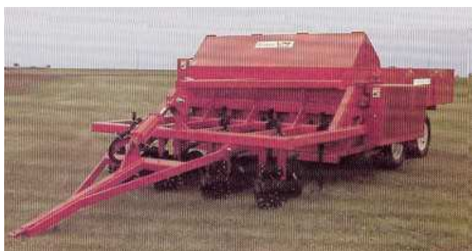
Front view: showing special coulters to cut thru residues.
