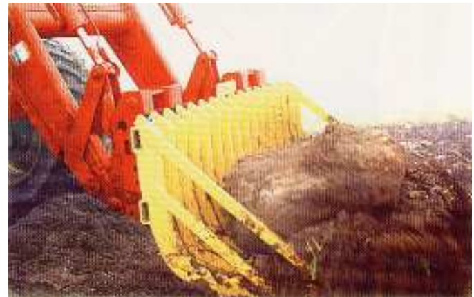
Rock Buckets: 4" spacing between teeth. Soils slip away thru the spacing between teeth, and rocks remain. 5 to 8-ft width.
