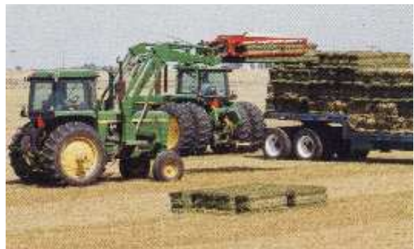
Bale Forks: Quickly picks up accumulated bales. Attaches to tractor front loader or skid steer loader.
