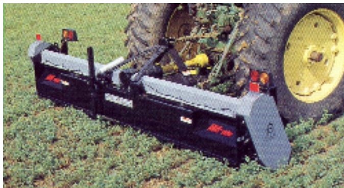
AGRI-vator: Pasture renovator, Track Conditioner. Vibrating tines fracture compacted soil on pasture and tracks.
