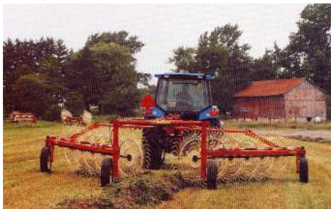
Hay Wheel Rakes: Gathers hay windrows together before harvesting. Bi-folds hydraulically or manually. Hi-capacity models have higher clearance for heaviest crops to pass through.
