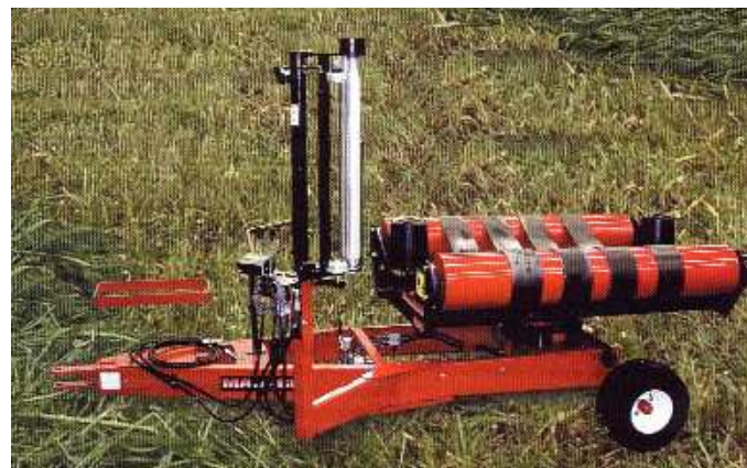
Round Bale Wrapper: Wraps bales up to 60" diameter. Self-loading arm, automatic cut, hand held remote control.
