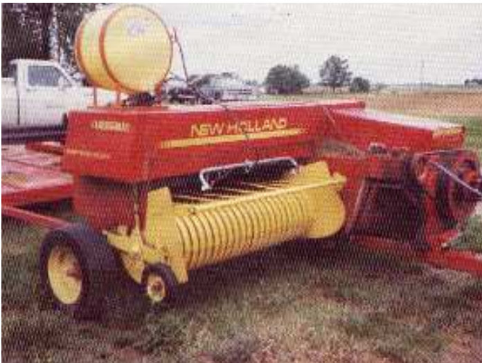
Hay Preservative Sprayers: Applies liquid preservative during baling or harvesting. 3 nozzle boom covers pick up width on baler. Optional In-Cab control for adjusting pressure from cab.
