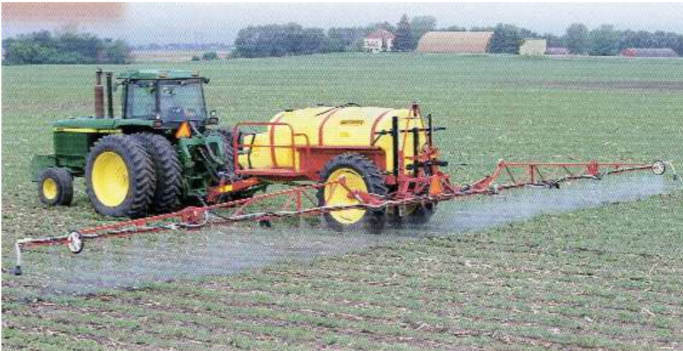
Large Row Crop Trailer Sprayers: 300 to 1000 gallon capacity elliptical tank. 45 to 60-ft truss boom. 18 or 20" spacing nozzles. Hydraulic lift & fold wings. Raven control. Roller pump or centrifugal pump. Optional foam marker, hand gun, Raven GPS light bar.
