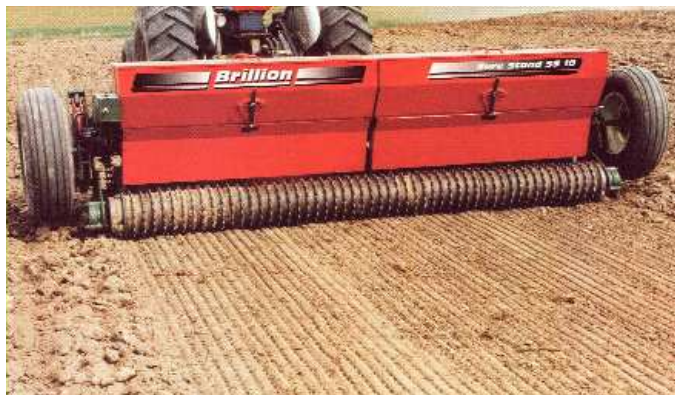
Grass Seeders: Plants alfalfa & other grass seeds. Grass will cover whole surface (not just rows). All seeds planted at 1/2" depth for maximum germination rate. 6 to 12-ft width models.
