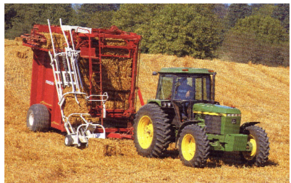
Bale Pick-up Wagon: Picks-up and stacks 56 to 77 bales. Unloads bales in block stacks for easier re-handling.
