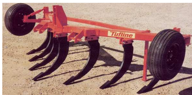
V-Plows: Breaks up hardpan and compaction. 28 or 32" shanks. 3 to 11 shank models. For 60 to 240-hp tractors.
