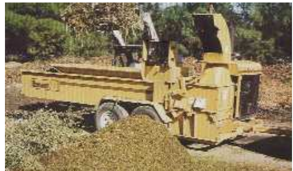
Mini Grinder: Grinds variety of wood wastes (tree branches, palm fronds, pallets..) to small particles. Hammermill action.
