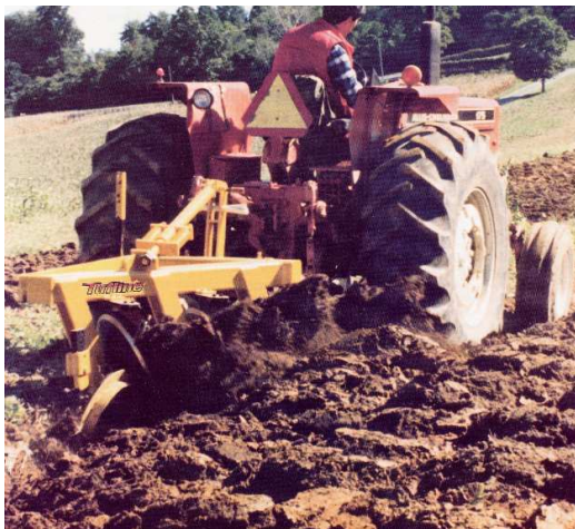
Disc Plows: 22 to 28" blades. For 40 to 65-hp tractors.
