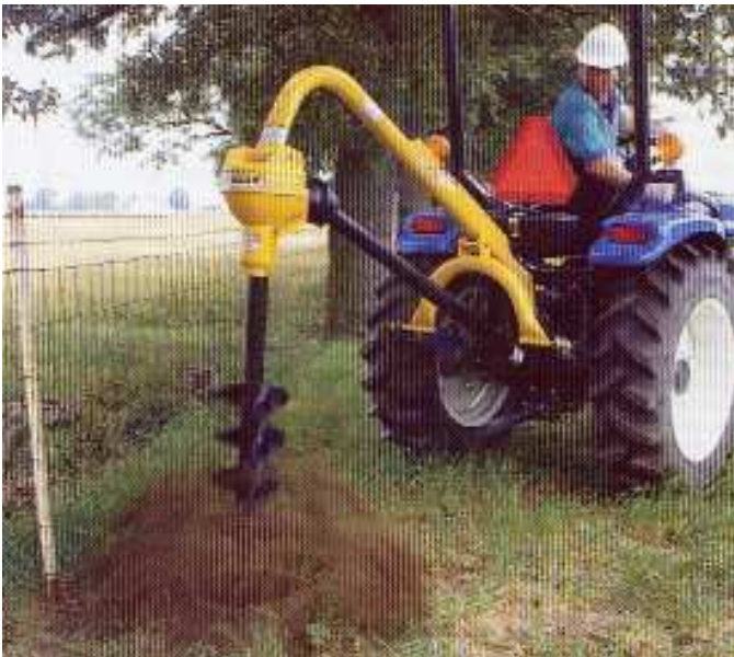
Post Hole Digger: PTO drive, 3-pt hitch mount. Also available: hydraulic drive front loader bucket mount, skid steer loader mount, backhoe dipstick mount and excavator dipstick mount.
