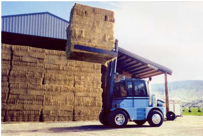
Roadrunner: Bale Stack Handler. Rapidly transports hay by the stacks for short or medium distances; between hay fields, stacking sites, truck loading sites and nearby dairy farms.
