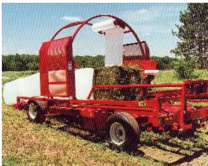
In-Line Bale Wrapper: Efficiently wraps round bales or big square bales one after another. Automatic & self-propelled.
