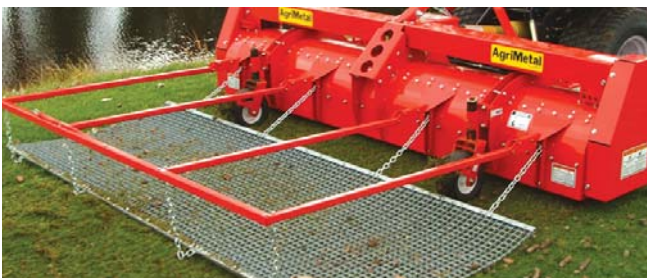
Core Breaker: breaks-up aeration cores; 1.8 or 2.4-meter working width; rotating rubber fingers break-up cores against stationary blades; steel drag mat spreads residue soil evenly.
