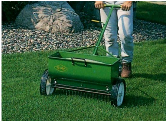
Small precision Drop Spreader: 61cm width; 5cm width semi-pneumatic tires; precision cam gauge metering.
