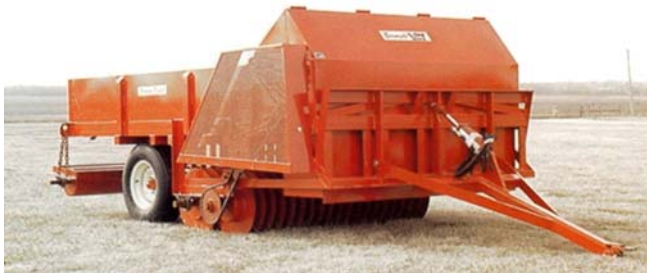
Sprig Planter: 2 to 6 row planters; 2 to 6 row no-till planters; or 1.2, 1.8, 2.4, 3.1-meter broadcast planters; ground-drive; coulter discs & rollers.
