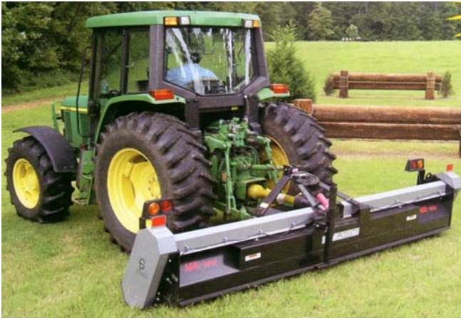
AGRI-vator: vibrating aeration system with deep tine penetration for horse racetrack renewal and soil renovation.
