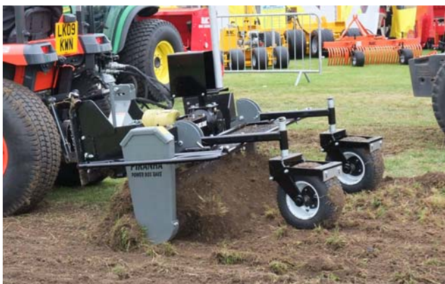
Power Rake: to prepare ground for seeding. Breaks up earth lumps, fluffs soil and spreads evenly.
