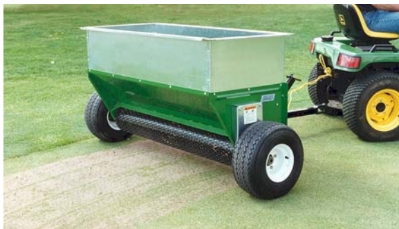
TruFlow tow-type Topdresser: lost-cost topdresser for dry flowable sand. 90 or 135-cm spreading width.
