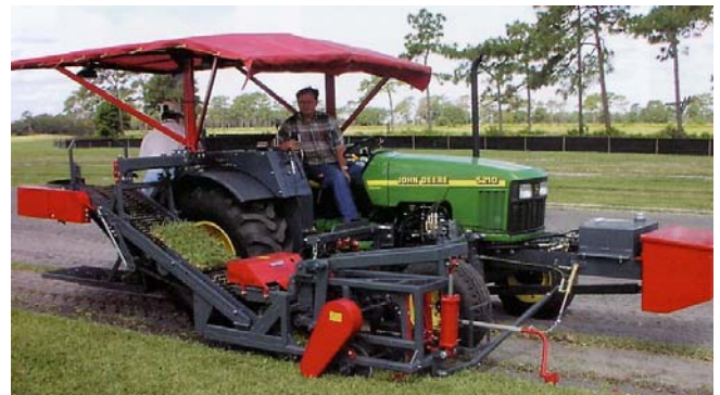
Sod Harvester: cuts 40, 46 or 60cm width; complete w/John Deere tractor; slabs or rolls; floating cutter head; hydraulic depth control; optional auto-steer.
