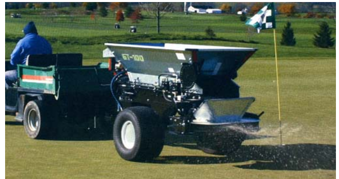
Precision Topdresser: tow-type; 9-hp Honda; adjustable spread pattern, depth & speed; dual 18" spinners; spinners tilt up/down 15° for light or heavy topdressing; 0.82 cubic-meter hopper; spreading width - up to 9.1-meter.
