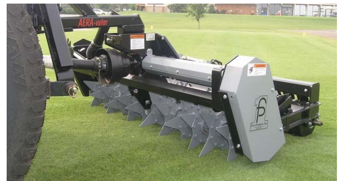
AERA-vator: Slicing Knives option easily installs instead of vibrating tines and makes no disturbing slices into short cut lawns and Bermuda grass.
