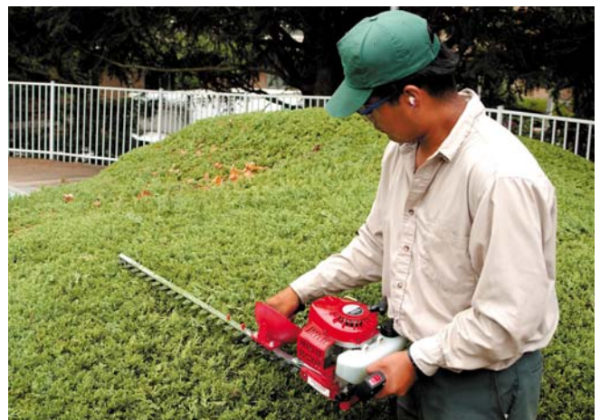
Hedge Trimmer: gas or electric; double sided or single sided blade; 50 to 76cm long blades; double activated switches for safety.
