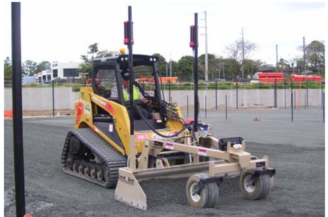
Laser-guided Leveling System: for all skid steers. Levels sports fields and green areas in general.
