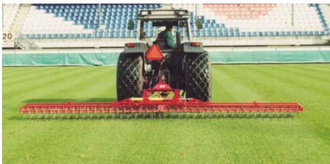
Large Area Dethatching Harrow with vibrating tines. Fast and easy system for frequent application to remove dead grass.
