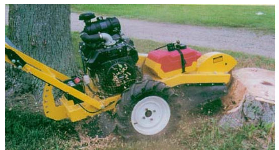
Stump Grinders for small or large operation eliminate stumps rapidly and safely. Choice of 12 to 20-hp engine.
