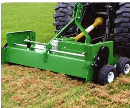
Dethatcher: PTO-drive w/slip clutch protection 1.22-meter width 20cm diameter sawtooth blades - 5cm blade spacing Overseeder attachment available
