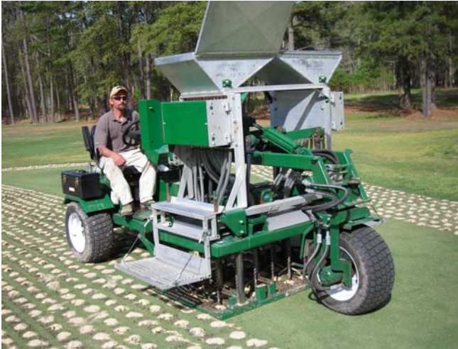
Drill & Fill Aerator: drills holes up to 30cm & fills same holes with sand; ideal for drilling through hard pan solving most drainage problems.
