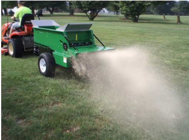
Affordable Topdresser with professional results. tow-type; hydraulic-drive; 4 tires; spreading width 0.9 to 1.8-meter; 0.8 cubic-meter hopper.
