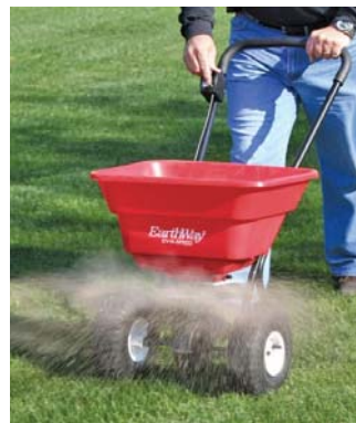
Commercial Broadcast Spreader: 45-kg or 25-kg poly hopper; pneumatic tires.
