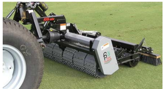
AERA-vator equipped with Multi-Tine System for artificial surface maintenance. Short tines aerate and fluff up plastic grass and even out rubber granular in artificial turf.
