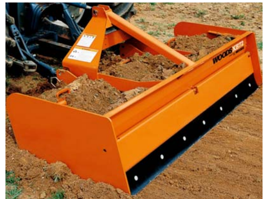
Box Scraper: tractor-mounted; 120-200cm width; Fixed, retractable or hydraulic scarifier bar.
