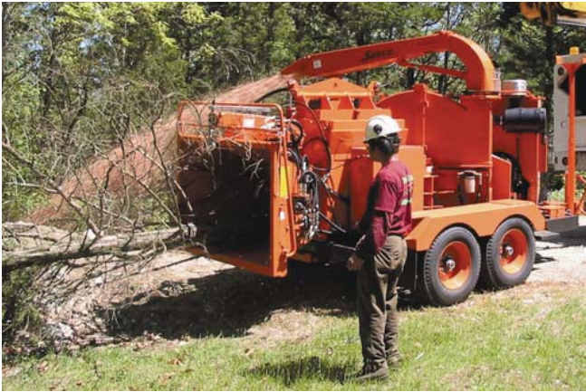
Selection of several sizes of Wood Chipper for commercial applications. Handles trees up to 18" (45cm) diameter powered by 225-hp diesel engine.
