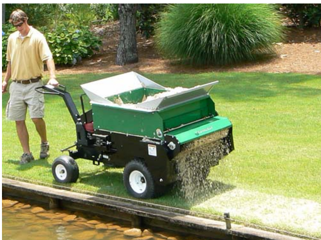
Self-propelled Topdresser: 10.5-hp B&S; hydrostatic-drive; 0.3 cubic-meter hopper; 76cm width brush.
