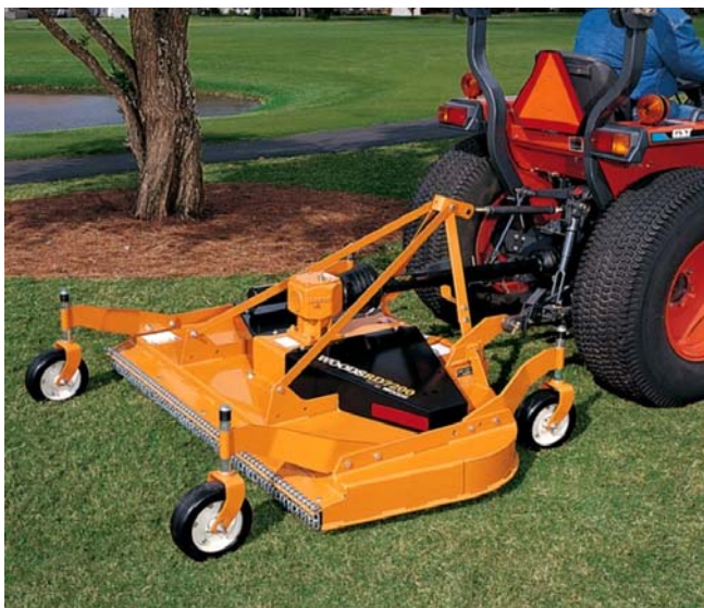
Finishing Mower: PTO-drive; 1.2 to 2 meter cutting width; side discharge or rear discharge.
