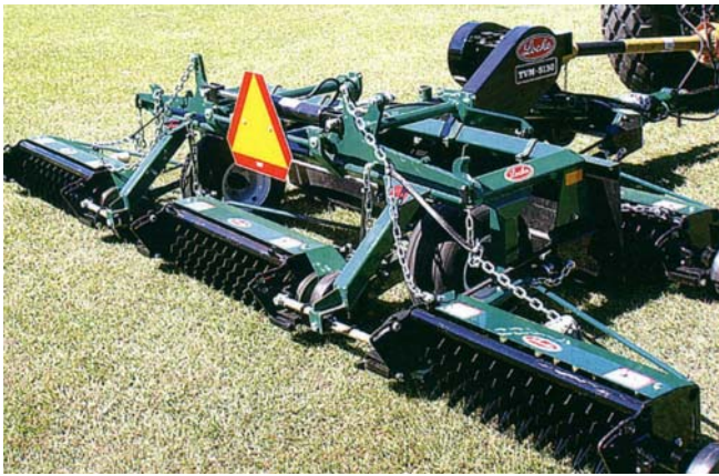
Gang Verticutter: PTO belt-drive; 2 to 3.3-meter width; cutting depth 0 to 2.5cm; 25cm diameter blades; hydraulic-folding wings, transport tires.
