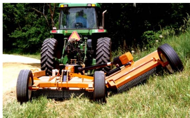
Offset Rotary Mower: PTO-drive; ideal for road-side maintenance; hydraulic folding wing; 3.2-4.3 meter width.
