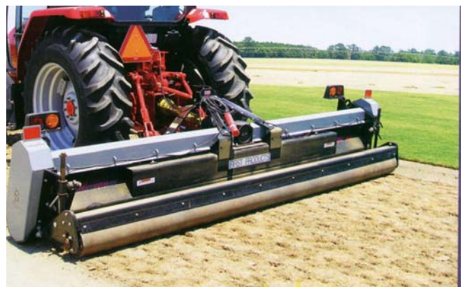
AGRI-vator: aerates / loosens soil before seeding; renovates root system to permit new seeding with less seeds; 15cm deep vibrating tines.
