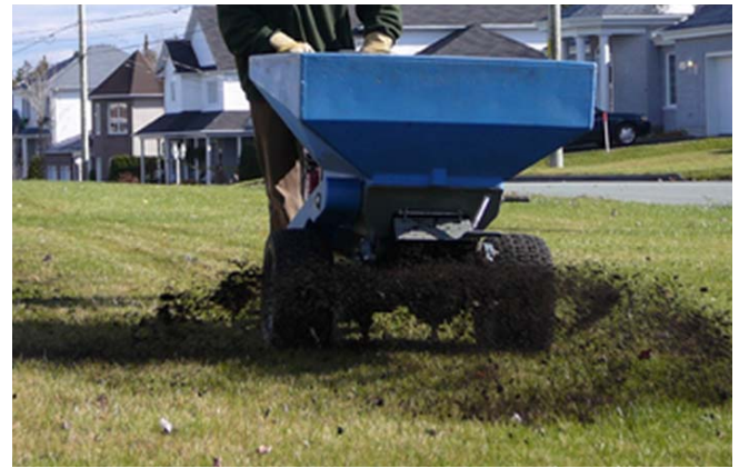
Self-propelled Topdresser: 5.5-hp Honda; 0.33 cubic-meter poly hopper; highly maneuverable; can spread top soil, compost, organic fertilizers, lime, sand.
