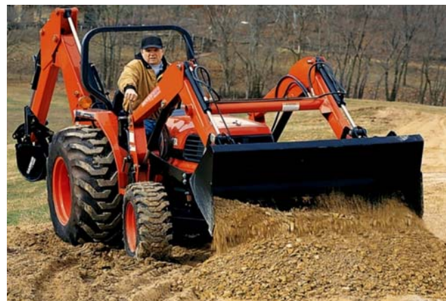
Front Loader: tractor front-mounted; joystick control; fits variety of tractors; variety of loader attachments also available.
