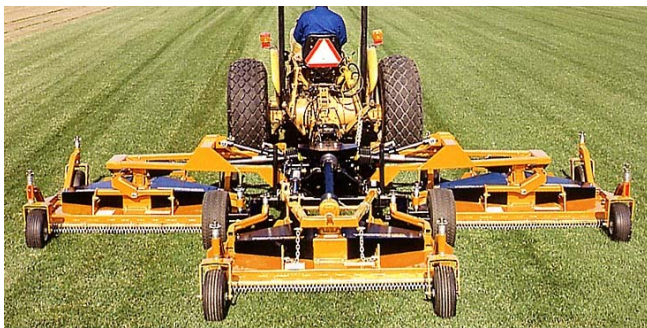
Wide Area Rotary Mower: tow-type; PTO-drive; hydraulic folding wings & transport tires; cutting width 3.7, 4.6 or 5.2-meter; 3 floating decks.
