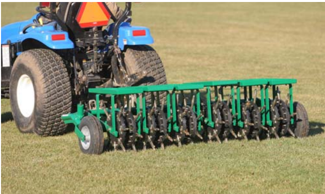
Ryan Renovaire Aerator: tow-type; designed to follow ground contour - each wheel pair is independently mounted; ideal for undulating turf areas.
