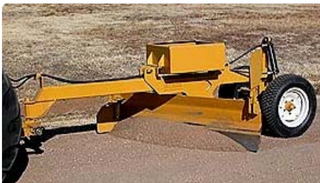
Compact Grader: tow-type; 180-250cm width; hydraulic blade angling (left /right); hydraulic tilting (one side up/down); ideal for undulating surfaces.
