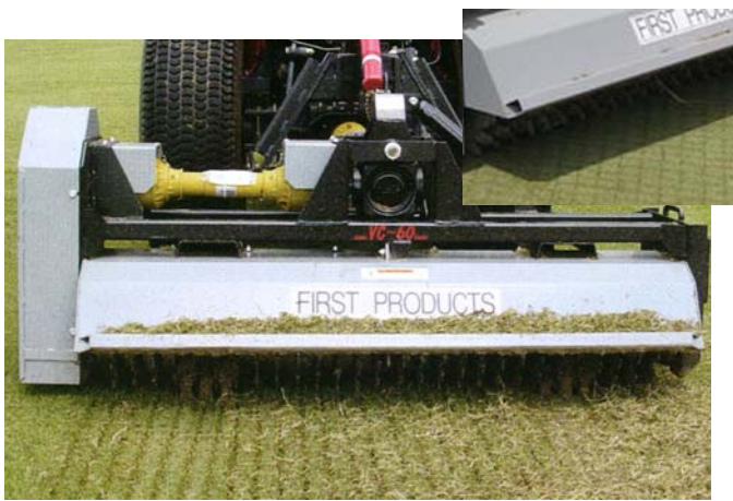
Verticutter: PTO-drive; 1.5-meter width; 30.5cm diameter blades; 5cm spacing; adjustable depth guides.
