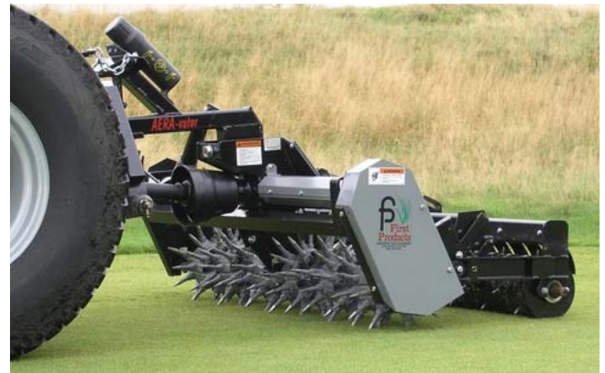
AERA-vator: vibrating aeration system shatters ground with vibrating tines. Especially designed for dry and very hard soil. No need to wet the ground before aeration.
