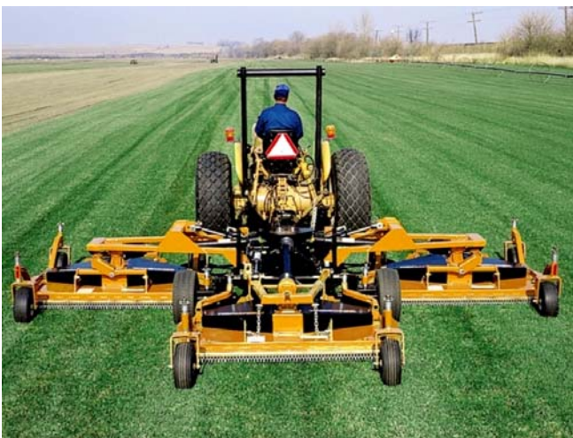
Wide Area Rotary Mower: folding wings; PTO-drive; 3.7, 4.6 or 5.2 meter width; ideal for sod farms.
