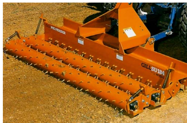
Landscaping Pulverizer: tractor-mounted; 120-200cm width; front spikes break up soil; rear rollers press down to make ideal seedbed.
