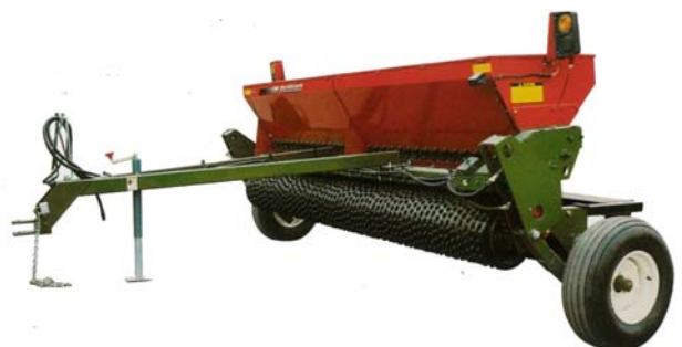
Turf Grass Seeder: tow-type; ground-drive; 1.8 to 3.66 seeding width; seeds are broadcast consistently at 1/2" depth for highest germination & seed savings.
