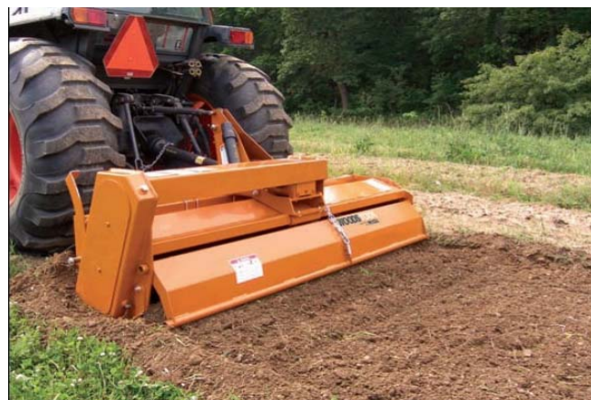
Rotary Tiller: PTO-drive, tractor-mounted; slip clutch; 5-9 flanges; 20-36 bearings
