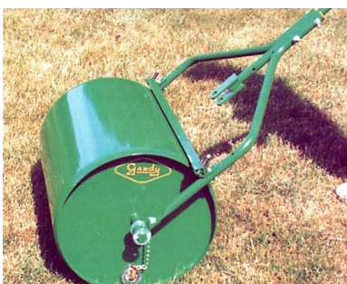
Gang Lawn Roller: tow-type; 1.8 or 3.6-meter width; steel rollers; water-fillable; foldable.
