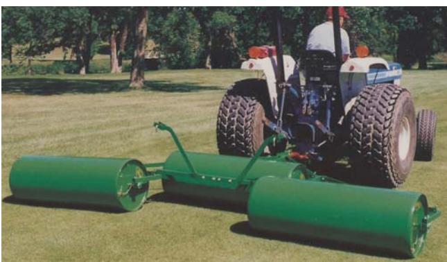
Gang Lawn Roller: tow-type; 1.8 or 3.6-meter width; steel rollers; water-fillable; foldable.
