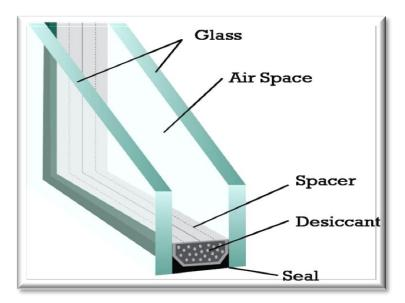
**Insulating glass** (IG) consists of two or more glass plies separated by a spacer to reduce heat transfer across a part of the building envelopes. Insulating glass units are sealed with a primary seal and a secondary seal of silicone. Unisunda offers multiple configurations of insulating glass units.
