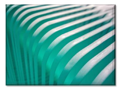
**Tempered glass** (also known as Toughened glass) is a type of safety glass processed by uniform heat treatment to increase its mechanical strength and thermal impact strength compared with normal glass. Tempering puts the outer surfaces into compression and the interior into tension. Such stresses cause the glass, if fractured, to shatter into small, relatively harmless granular chunks.
