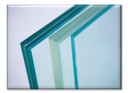
**Laminated glass** is a type of safety glass produced by bonding two or more layers of ordinary annealed or tempered glass together with one or more interlayer(s). When broken, numerous cracks appear, but glass fragments tend to adhere to the interlayer.
