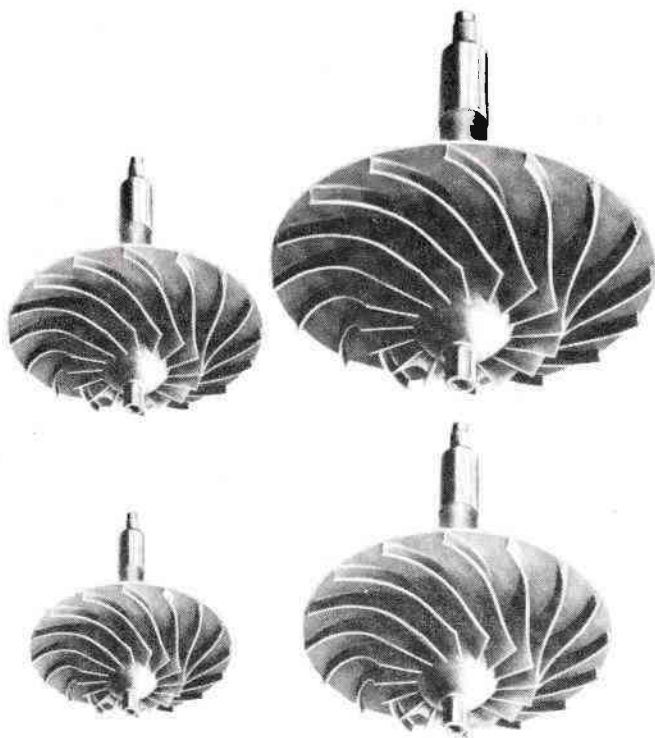
Fig. 1-9—Investment cast stainless steel (17-7PH) impellers having back-lay vanes and without a shroud. The performance for a similar impeller is shown in Fig. 1-5. (Courtesy of Chicago Pneumatic Tool Co.)
