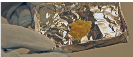
Fig. 77. To perform a crackle test, first put the grease sample on a piece of aluminum foil.
