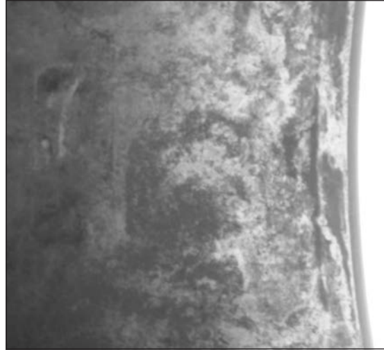
Fig. 47. Classic fretting corrosion from poor fitting practice is depicted here. Relative movement under load between the bearing and its seat caused this worn and corroded condition.
