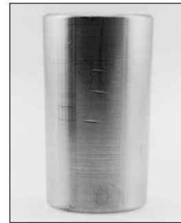
Fig. 39. Rough handling or installation damage resulted in nicks and dents in this tapered bearing roller.
