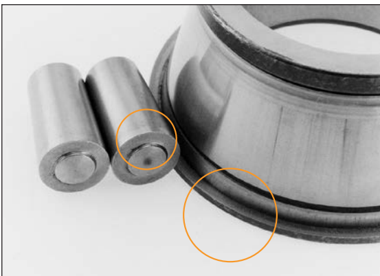
Fig. 3. Fine particle contamination caused abrasive wear on this tapered roller bearing.
