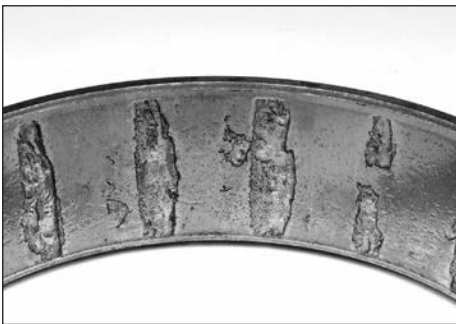
Fig. 14. Advanced spalling initiated at water etch marks on the cup race makes this bearing unsuitable for further service.
