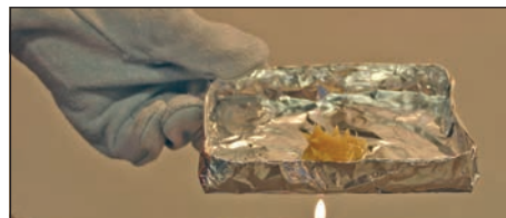
Fig. 78. A crackle test determines the presence of water in grease.
