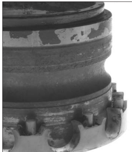
Fig. 15. Heavy water damage is shown on this ball bearing inner ring and cage.
