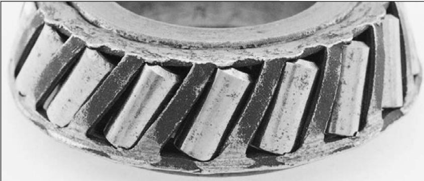
Fig. 44. Binding and skewing of these tapered rollers was due to compression of cage ring during installation or interference during service.
