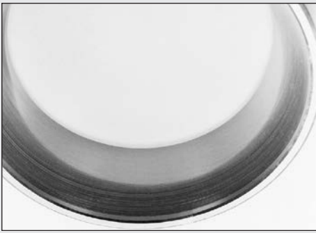
Fig. 36. Deflection, inaccurate machining or wear of bearing seats caused an irregular roller path on this tapered roller bearing outer ring.
