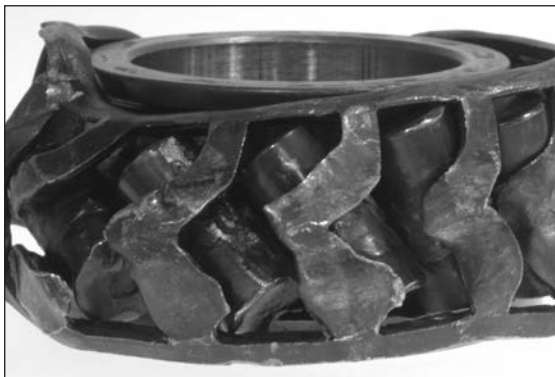
Fig. 22. Level 4 – This is an example of total bearing lockup.
