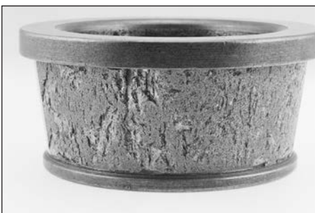
Fig. 29. High loads and low speeds caused insufficient lubricant film on this tapered roller bearing cone.
