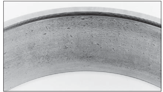
Fig. 7. Debris from other fatigued parts, inadequate sealing or poor maintenance caused bruising on this tapered roller bearing race.
