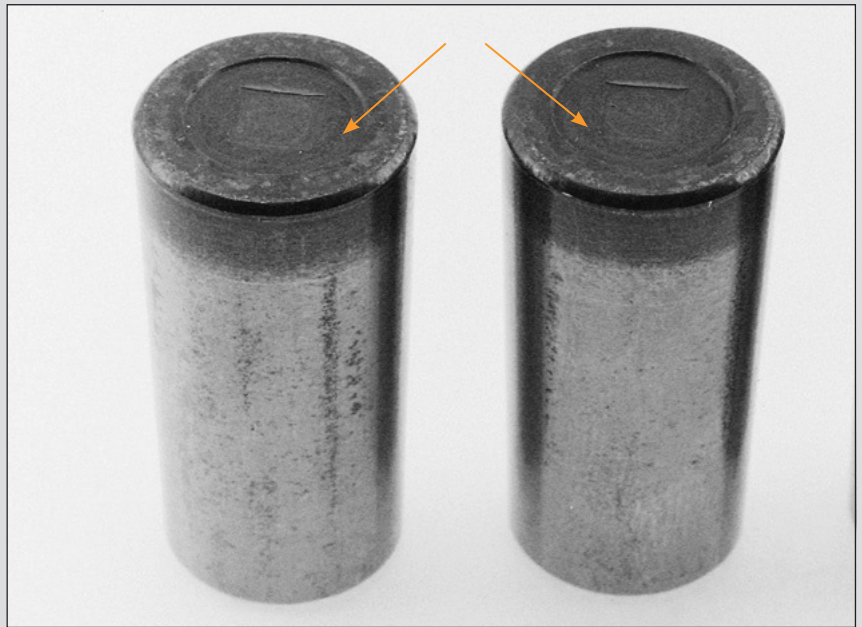
Fig. 20. Level 3 – Heat damage on these tapered rollers was caused by metal-to-metal contact.
