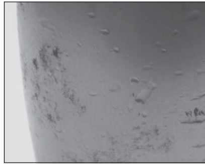
Fig. 6. Hard particles caused contamination bruising on this spherical roller bearing.
