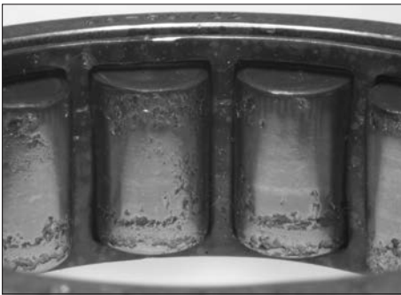
Fig. 26. High loads resulted in fatigue spalling on this cylindrical roller bearing.
