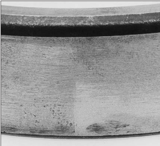
Fig. 48. The marks on the outside diameter of this cup are caused by a high spot on the housing. The cup race is spalled at the spot that corresponds to the spot on the outside of the cup marked from heavy contact.
