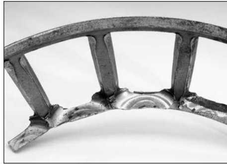
Fig. 33. Cage pocket damage results from excessive roller movement.
