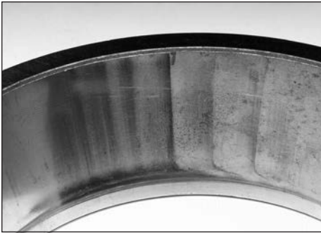
Fig. 32. Scalloping marks in the cup are common with excessive endplay. This occurs when unloaded rollers enter the small load zone and are suddenly exposed to heavy loads.
