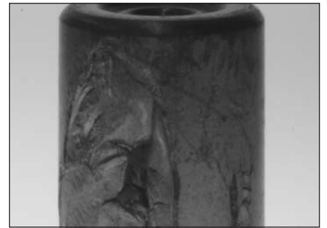
Fig. 28. Overloading on this cylindrical roller bearing caused roller surfaces to fracture.
