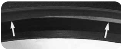
Shaft-to-bore misalignments (left) and dynamic run-out (right) both cause early lip leakage (fig. 9d).
