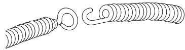
The hook and eye provides positive spring connection on seals for larger (18" diameter) shafts (fig. 8l).
