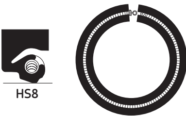
Connect the split seal's spring after the seal is placed around the shaft (fig. 8i).
