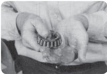
To lubricate the bearing, force grease around the outside of the bearing and between internal parts. (fig. 3)
