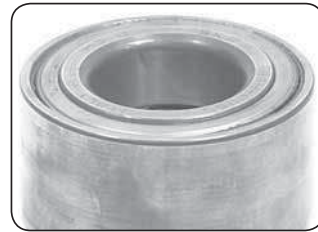
Seal in an oblique position due to wrong fitting during mounting into the knuckle.
