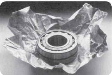
Wrap the bearing in waterproof paper. (fig. 10)
