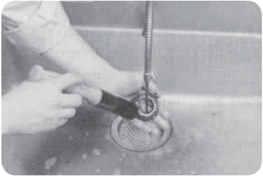
Rinse the bearing in clean solvent. (fig. 7)
