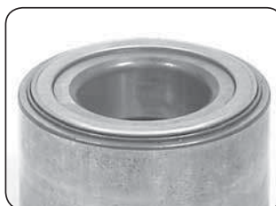
Seal standing out from inner and outer ring due to wrong fitting.
