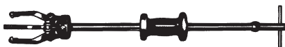
Slide hammer pullers, which can remove parts from blind holes, also may be used to remove the bearing. (fig. 4)
