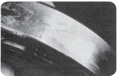
Fretting occurs when excessive friction causes metal particles to break off the bearing race. (fig. 3)
