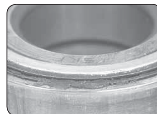
Detail of picture at left showing grease leakage.
