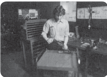
The work area should be clean before you take the bearing out of its package. (fig. 2)
