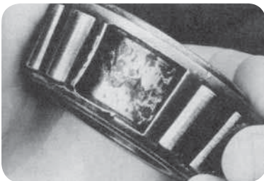
Spalling begins as small fractures under the bearing's surface. (fig. 5)
