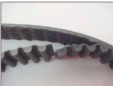
Figure 8 – Tooth separation failure
