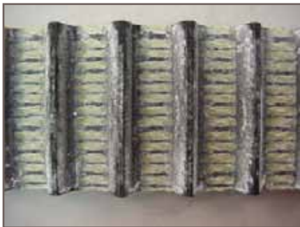
Figure 16 - Extreme wear from abrasion
