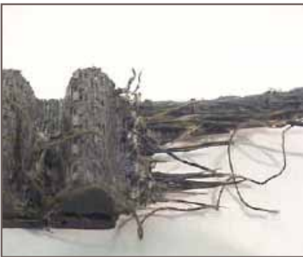
Figure 4 – Typical shock load failure
