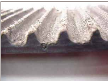
Figure 9 – Excessive tooth wear
