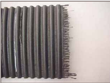
Figure 20 - Crimp failure due to debris
