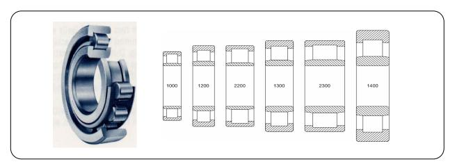
For each size there are many configurations (types) as shown below. The type depend on the ribs on the inner and outer ring. The most common types are the NU and NJ. NU has two ribs on the outer ring and no ribs on the inner ring, this type can not accept thrust load. The NJ has two ribs on the outer ring and one rib on the inner ring, this type can accept thrust load in one direction.
