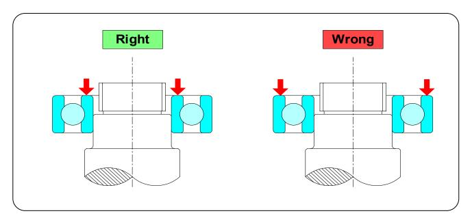
When force is to be applied on the rolling bearing for mounting, it must be applied in a straight line and evenly. Make sure that bearing is centered correctly.
