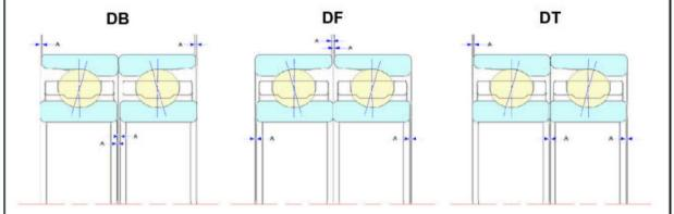
These sets of two bearings have been selected as matched pairs at the factory. One DU set of bearings has only a small dimensional variation (2 µm maximum) on the bore diameter and OD of the two bearings. The Dimensions are shown on the inspection sheet in the box and on the side of the box. Each bearing is serialized.
