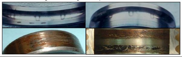
**Smearing:** Metal to metal contact due to the destruction of oil film.
