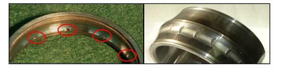
False Brinelling: The occurrence of elliptical wear at ball or roller spacing
