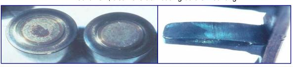
Rusting, Corrosion: Rusting and corrosion is oxidation of the steel. Can cause
