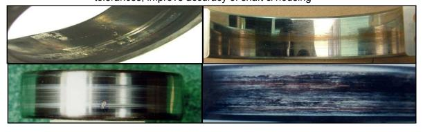
**<u>Electric Arcing:</u>** Pitted or corrugated surface caused by electric current pass.
