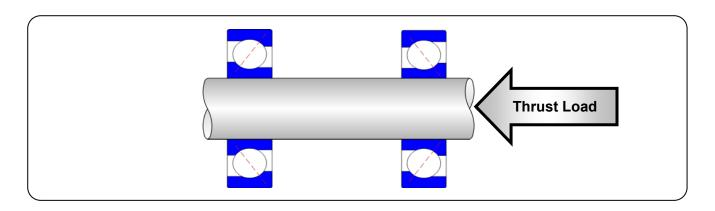
The "C" Capacity of the bearing is used to calculated bearing life. The loading ratio "load/C" indicates type of load. 1% to 8% are lightly loads, 8% to 18% medium loads; heavy load 18% to 25%, Light loaded applications tend to operate at higher speeds, medium loaded applications operate at half of the speed limit of the bearings, and heavy loaded application operate at low rpm.
