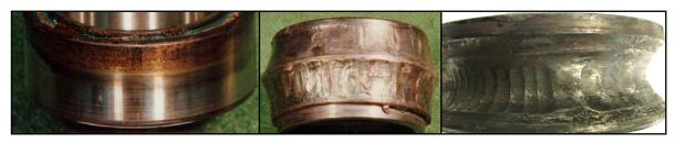
Flaking: Repetitive Heavy stress cycle between the bearing raceways and
