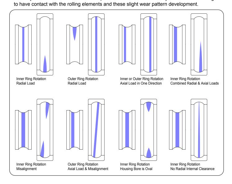
Bearings are like fuses, something causes the bearing to fail. We use these visual wear patterns to determine if the application is normal or if something is abnormal. By shinning a bright light (Mag flashlight) down the raceway these, patterns pop out and become more visible.
