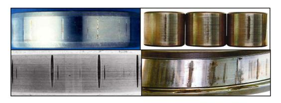
Fretting: It is the wear and oxidation due to repetitive sliding between
