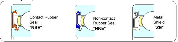
Nachi's design utilizes a groove in the inner ring and the seal contacts the side of the groove. Standard material for seals is Buna N (Nitrial Rubber).
