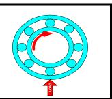
The shaft rotates and the direction of the load does not change. The outer ring is stationary. The entire inner ring raceway comes under load during one revolution of the shaft.
