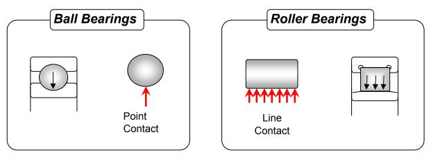
Bearings are divided into two groups Ball and Roller. The balls in ball bearings transfer the loads over very small areas with the raceways, we describe this as point contact. The rollers in roller bearings transfer the loads over larger areas with the raceways, we describe this as line contact.
