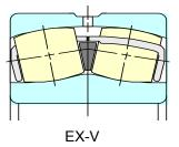
Vibrating Screen Bearings are special spherical roller bearings as the applications are most sever. We now can offer two bearings with different cages for this extremely harsh application. Our standard bearing with a machined bronze cage is coded AEX-V and our new high capacity bearing with the heat treated stamped steel cage is coded EXV.
