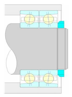
On "DF" arrangements a housing cover preloads the bearings.
