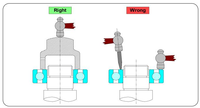
When you are mounting the inner and outer rings at same time, use a metal buffer and apply a force simultaneously on both rings.
