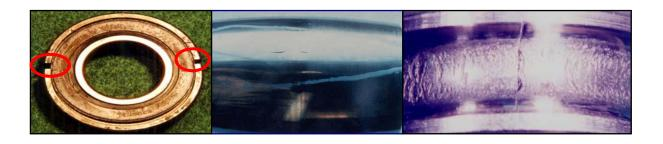
Fracture: Cracked inner ring rib. Broken retainer.
