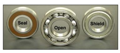
The capacity of a bearing will be the same regardless if it has seals, open, or shielded. All three bearings will accept the same load and produce the same life. The three bearing will have different speed limits. Speed limits are determined by how hot
