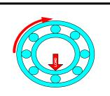
The shaft remains stationary and the outer ring rotates, The direction of the load does not change. The entire outer ring raceway comes under load during one rotation of the housing. Only a portion of the inner ring raceway ever comes under load.
