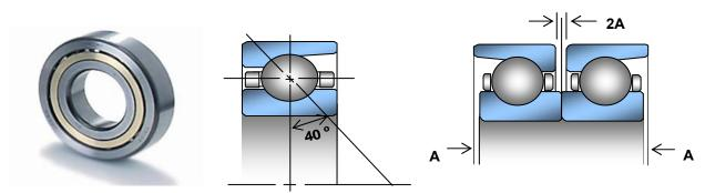
**BMU** bearing commonly referred to as thrust bearings can be used in pairs. The inner ring and the outer ring have identical widths. This permits the bearings to be arranged in any combination such as back to back face to face or tandem pairs. The 40° bearing angle enables the bearings to accept heavy axial loads.
