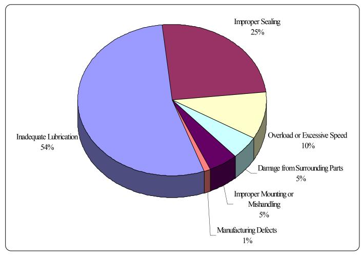
The majority of premature bearing failures are caused by inadequate lubrication. Anti-friction rolling element bearings are designed to have a thin film of oil between the rolling elements and the raceway surfaces. When this film degrades or gets too thin the rolling elements contact the raceway surfaces and wear develops. Anti-friction bearings are not designed to wear when bearing wear bearings wear out.
