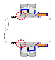
Periodically check the internal radial clearance. When the required reduction in radial clearance is measured advance the locknut to the align up the locknut to the closest lock washer tang and bend the tang over into the slot to secure the locknut from backing off.
