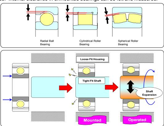
Country standards (ABMA, JIS, DIN) and international standards (ISO) for clearance ranges are the same. These clearance ranges will vary depending on type of bearing (Radial or or Angular) and (Ball or Roller)
