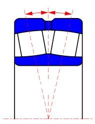
Double Row Spherical Roller Bearings are the work horse of the industry. Their Ball Shaped outer ring and Barrel Shaped Rollers permits this bearing to operate with misalignment with no reduction in bearing life. These bearings will operate and except static misalignment or dynamic misalignment with no reduction in life.
