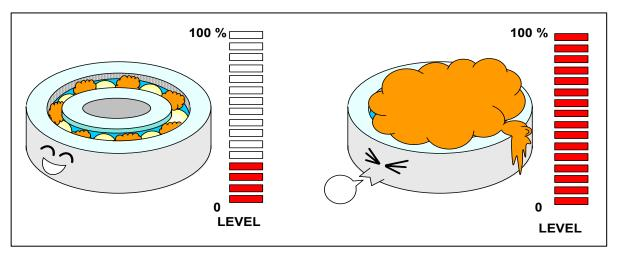
Nachi Standard grease fill for sealed and shielded ball bearings is 20% to 30% full
