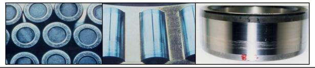
**Excessive Wear:** Surface deterioration due to heavy sliding friction between
