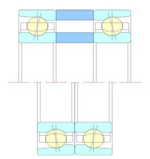
Bearings at free end are cylindrical roller bearings or bearings which are not fixed in the axial direction. Angular contact ball bearings at free end have loose fit and no shoulder on the housing or shaft. Therefore, they can have loose fit and no shoulder on the housing or shaft. Therefore, they can move in the axial direction and they do not carry axial load. The free end is also the expansion end.
