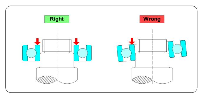
When a press is not available, hammer in the bearing, using only a dead blow hammer and a mounting dolly to minimize the shock to the bearing and evenly distribute the mounting forces. The bearing should not be hammered directly and pressure should be applied only to the inner ring.
