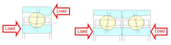
Single row angular contact bearings can only be loaded in one direction. If the bearing is loaded in the wrong direction away from the back face the bearing:
