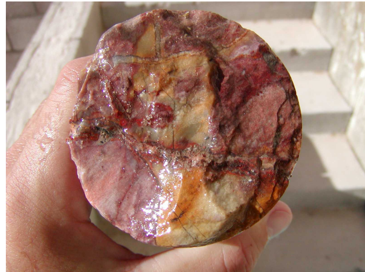
Breccia and veining in core showing strong alteration and iron oxide
