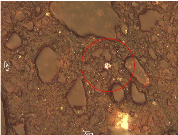
Small 5µm grain of Au in a matrix of iron oxide and granular quartz.
