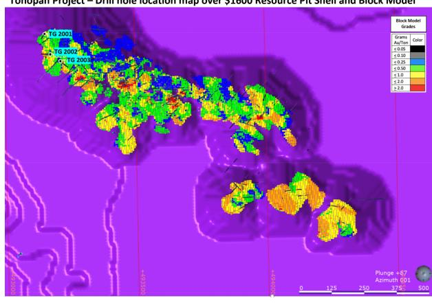
Tonopah Project - Drill hole location map over \$1600 Resource Pit Shell and Block Model
