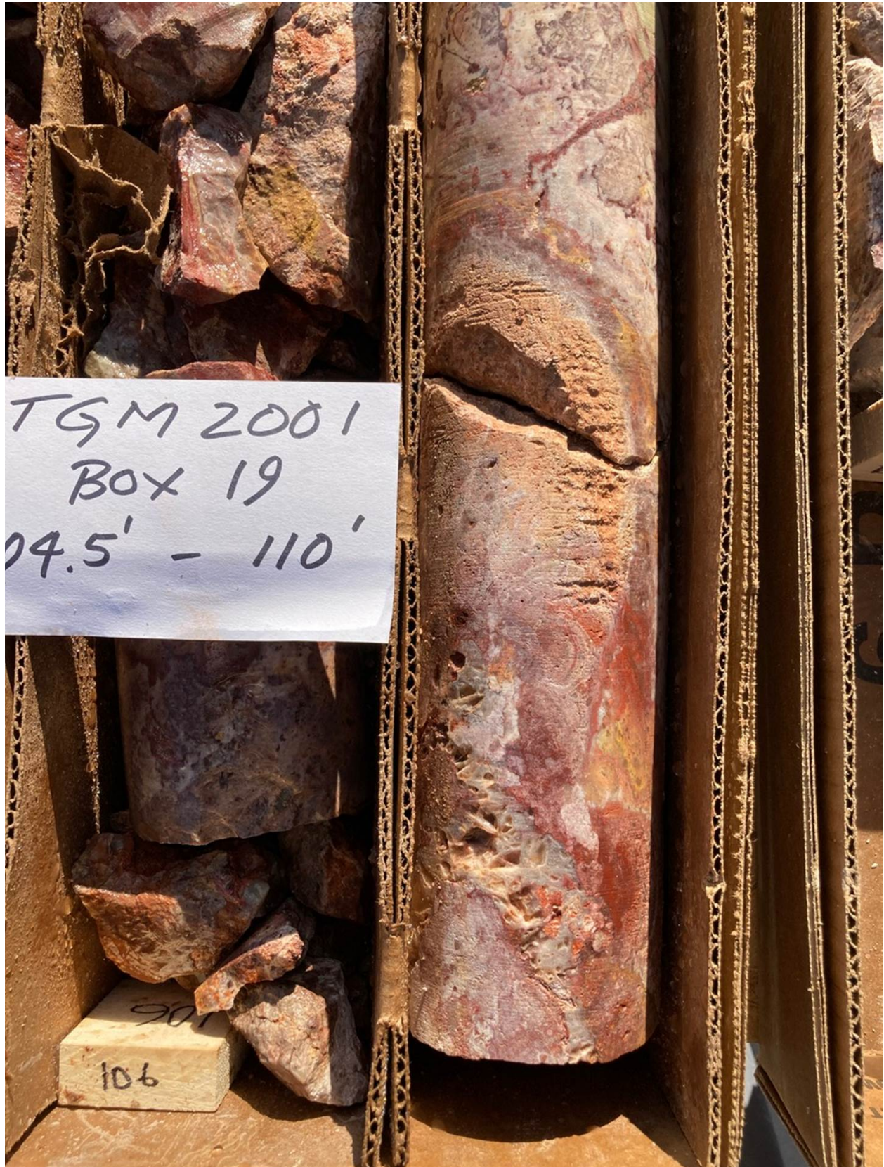
TGM 2001 – 85mm dia PQ core- Intensely silicified and oxidized tertiary volcanic with quartz veining
