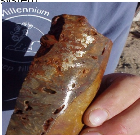
Drill core showing free gold
