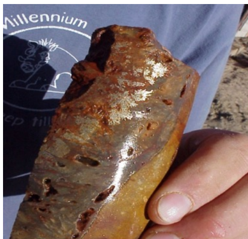
Drill core showing free gold
