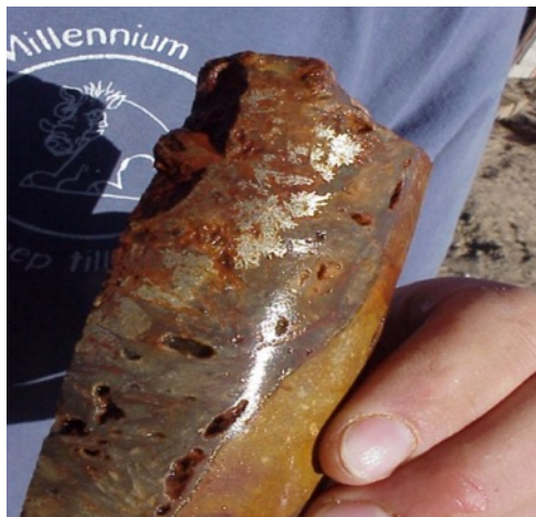
Drill core showing free gold
